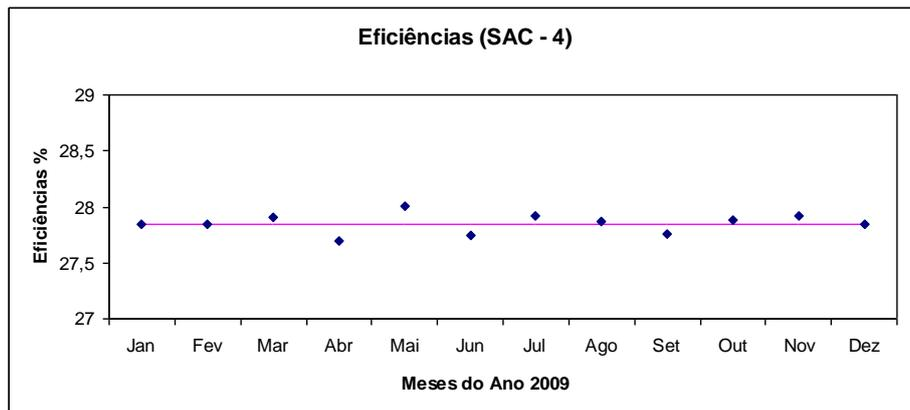
**Figure 4: Efficiency values for the alpha counter in 2009**
