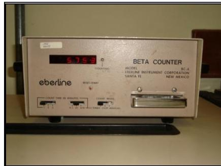
**Figure 3: Fixed Monitor (BC-4): beta counter**
