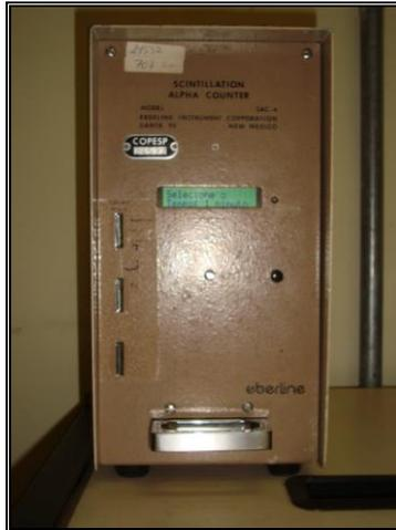
**Figure 2: Fixed Monitor (SAC-4): scintillation alpha counter**
