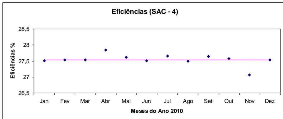
**Figure 5: Efficiency values for the alpha counter in 2010**
