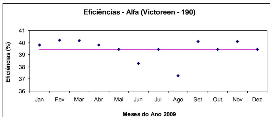
**Figure 7: Efficiency values for the Geiger-Muller monitor for the source emitting of alpha particles in 2009**
