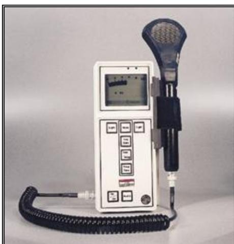
**Figure 1: Portable Monitor: Geiger-Muller with pancake probe type for the surfaces**
