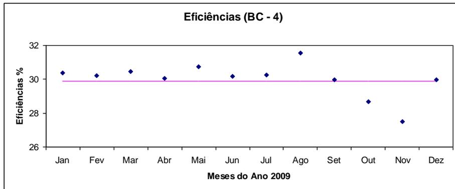
**Figure 6: Efficiency values for the beta counter in 2009**
