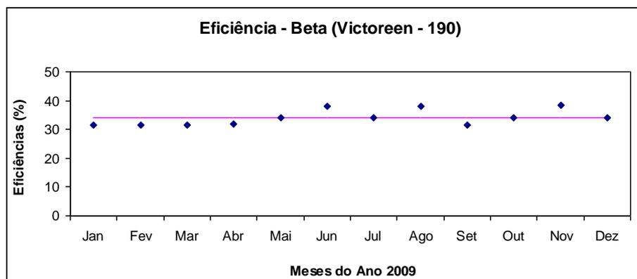
**Figure 8: Efficiency values for the Geiger-Muller monitor for the source emitting of beta particles in 2009**
