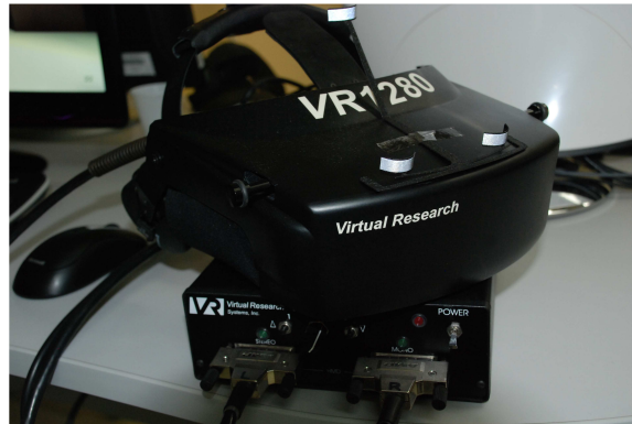
4.3.1 - HMD with IR reflectors.
