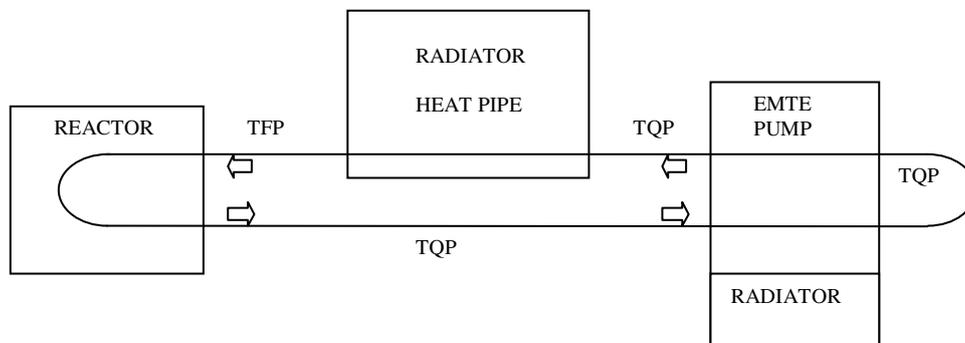
**Figure 5. Thermal hydraulic balance of SP-100 simulated.**
