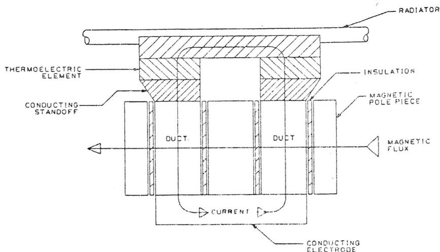
**Figure 3. Cross section of the EMTE pump.**
