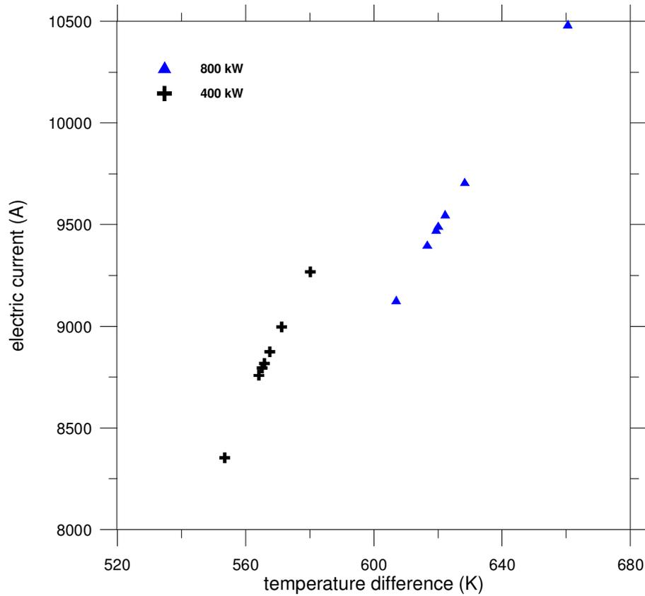
**Figure 7. EMTE pump electrical current.**
