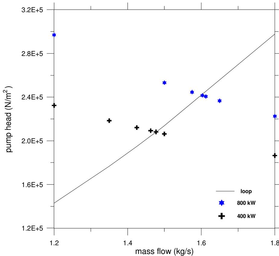
**Figure 9. EMTE pump curve for the SP-100 primary loop.**
