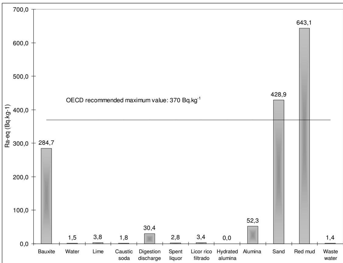
**Figure 2. Ra-eq for each sample compared to OECD limit for building materials.**
