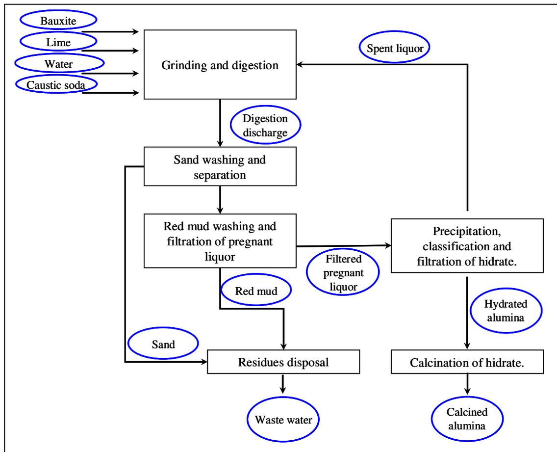
**Figure 1. Simplified fluxogram of Bayer process, including samples collected in each phase.**
