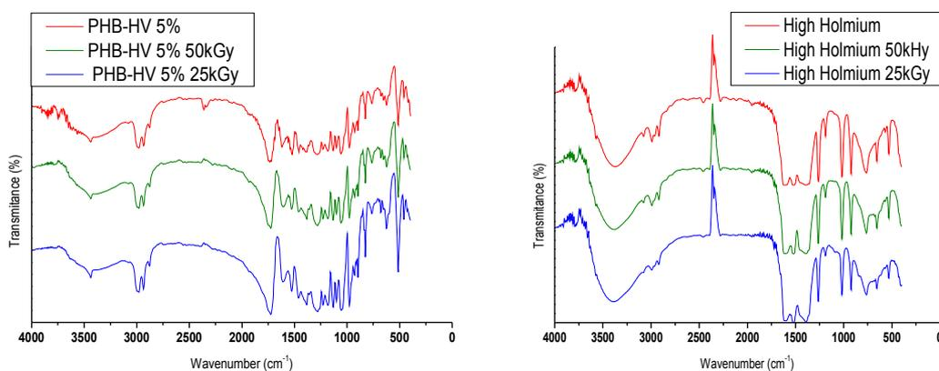
**Fig. 11 Infrared spectra of PHB-HV 5% and HoAcAc microspheres non-irradiated and irradiated at 25 and 50 kGy doses.**
