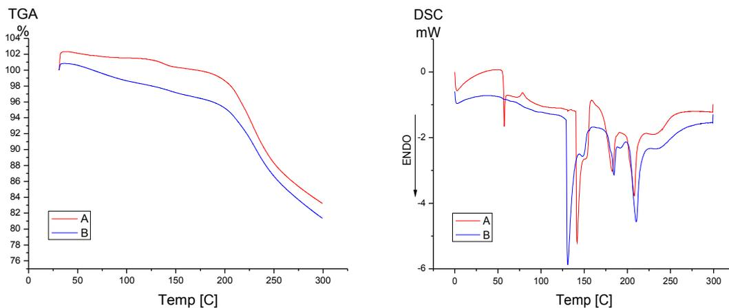
**Fig. 9.** TGA and DSC of HoAcAc microspheres (A) non-irradiated and (B) gamma irradiated with 25kGy.
