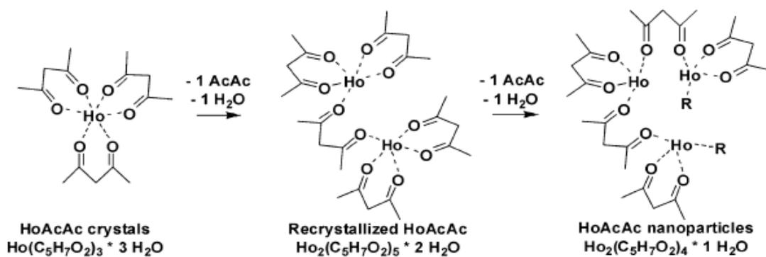
**Fig. 6.** Schematic representation of recrystallization of HoAcAc and formation of the microspheres. Adapted from Bult e col. 2010 (4)
