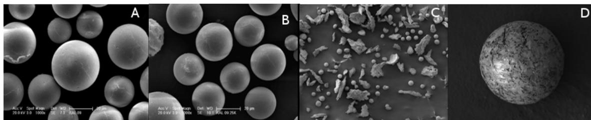
**Fig. 3.** A scanning electron micrograph of non gamma irradiated microspheres of High Holmium Content, B scanning electron micrograph of gamma irradiated at 25kGy microspheres, C and D scanning electron micrograph of microspheres after gamma irradiation at 50kGy (magnitude 500x and 1000x respectively).
