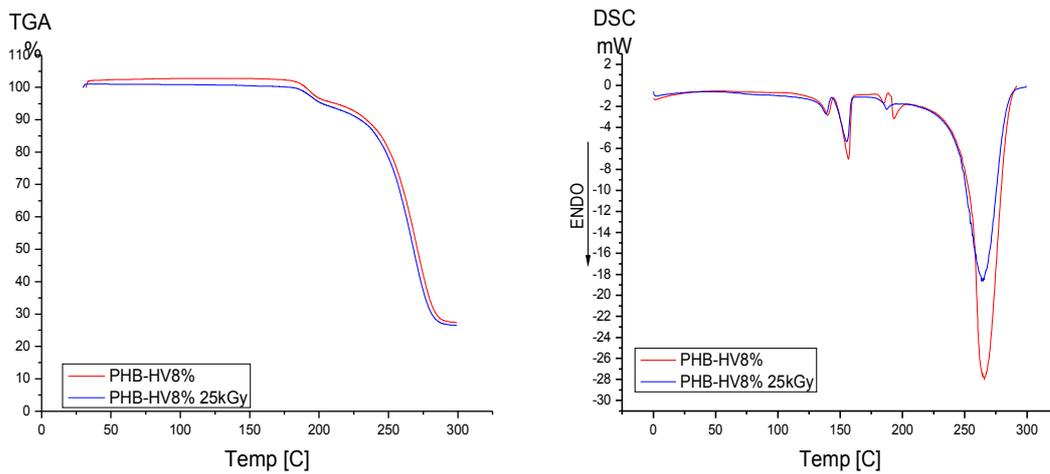
**Fig. 8. TGA (A) and DSC (B) curves of non-irradiated microspheres of PHB-HV 8% and gamma irradiated with 25kGy.**
