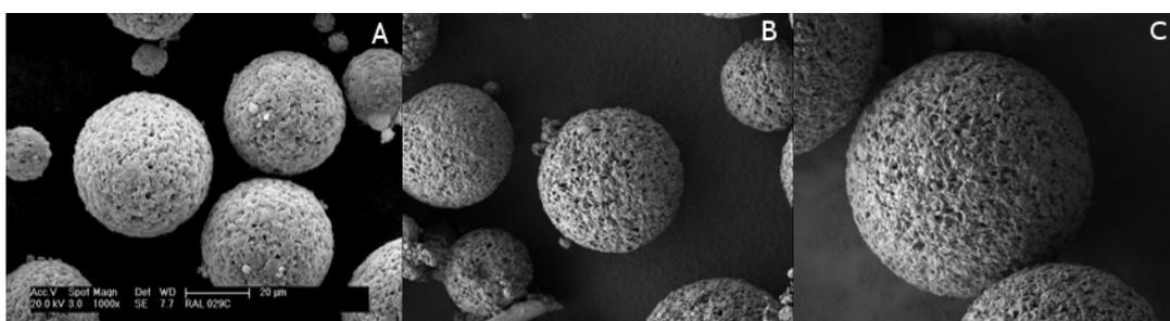
**Fig. 1. A scanning electron micrograph of non gamma irradiated microspheres of PHB-HV 5% of HV, B scanning electron micrograph of microspheres gamma irradiated 25kGy and C scanning electron micrograph of irradiated microspheres with 50kGy.**
