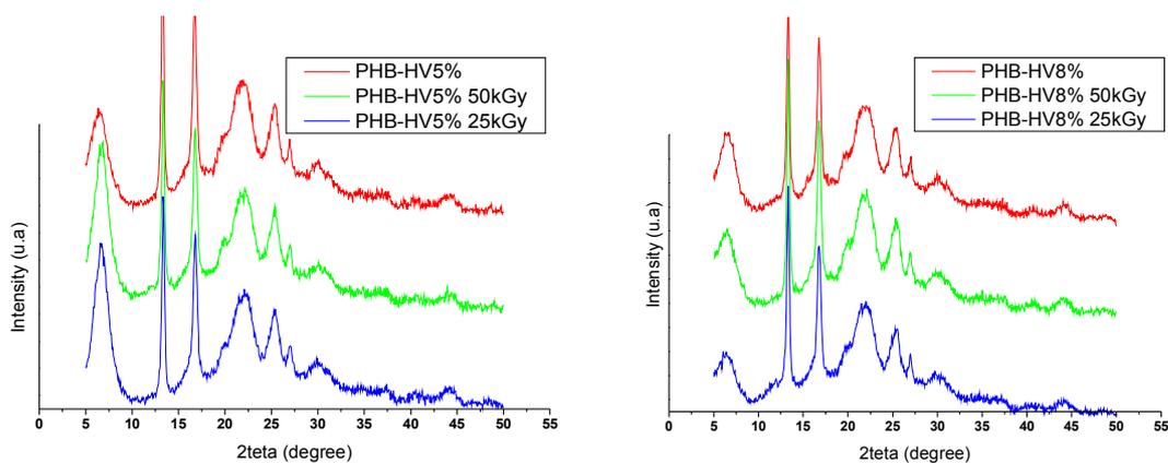
**Fig. 10 DRX spectra of PHB-HV 5% and 8% microspheres.**
