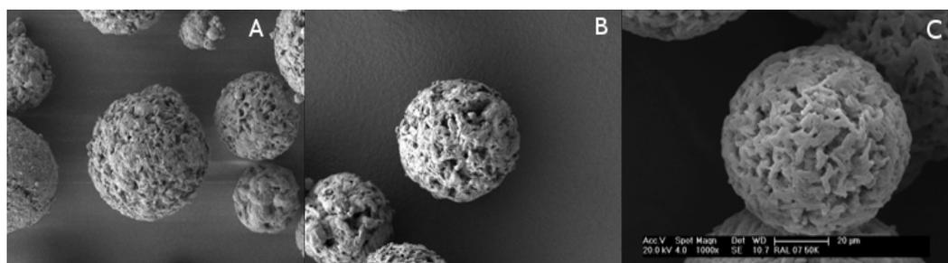
**Fig. 2. A scanning electron micrograph of non gamma irradiated microspheres of PHB-HV 8% of HV, B scanning electron micrograph of microspheres gamma irradiated 25kGy and C scanning electron micrograph of irradiated microspheres with 50kGy.**
