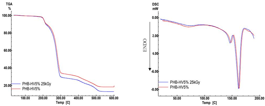
**Fig. 7. TGA (A) and DSC (B) curves of non-irradiated microspheres of PHB-HV 5% and microspheres irradiated with gamma 25kGy.**
