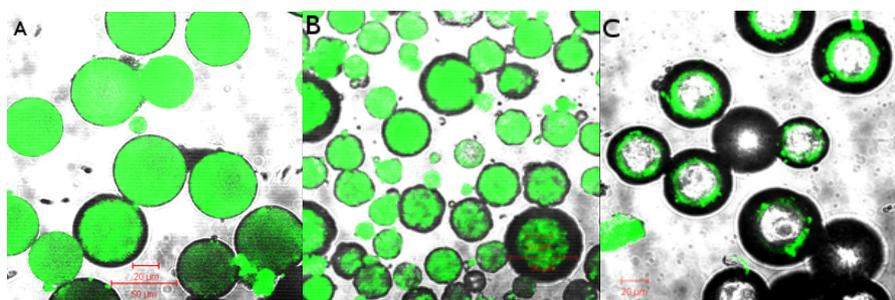
**Fig. 4.** CLSM images of A PHB-HV 5%, B PHB-HV 8% and C High Holmium Content microspheres.
