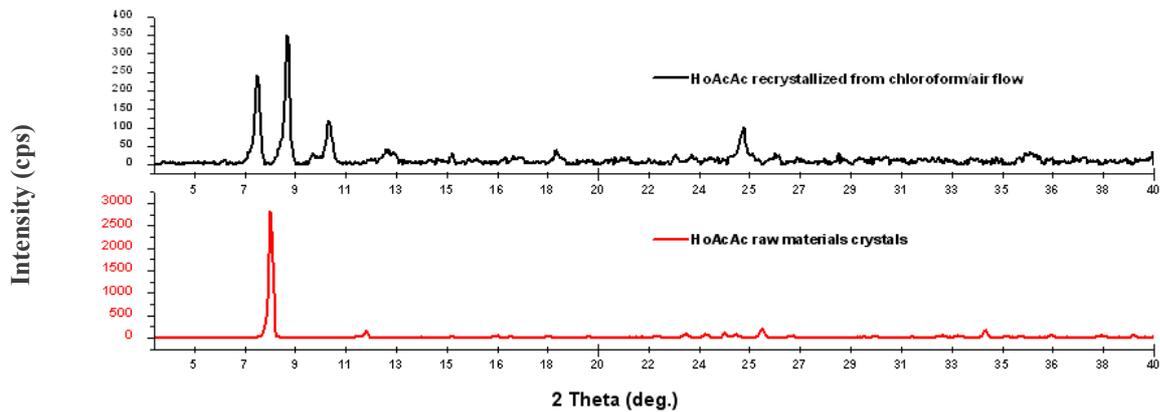
**Fig. 5.** X-ray scattered intensity as a function of the diffraction angle  $2\theta$  X-ray Diffraction of HoAcAc and HoAcAc recrystallized from  $\text{HCCl}_4$ .
