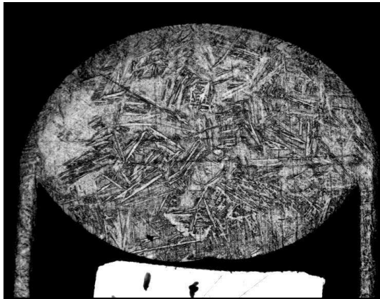
Figure 17. Titanium tube weld detail (125x).
