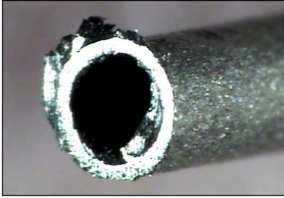
Figure 6. Titanium tube with burrs after cutting operation.
