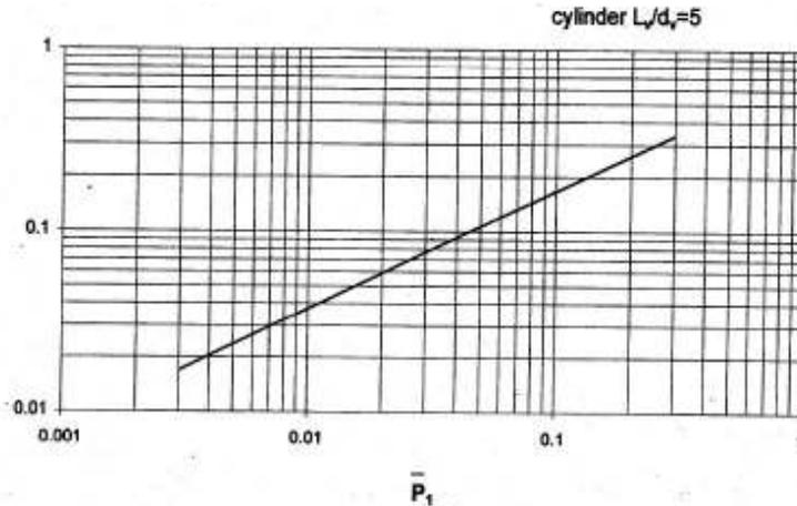
Figure 3 - Speed climbing fragment versus pressure for cylindrical vases containing ideal gas, where  $L_v$  and  $d_v$  are the height and diameter of the vessel, respectively [6]
