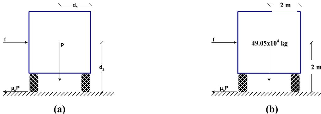
**Figure 2 - (a) Schematic of forces for the analysis of the possibility of truck overturning due to pressure caused by explosion of a H<sub>2</sub> cylinder. (b) - Dimensions of the tanker**
