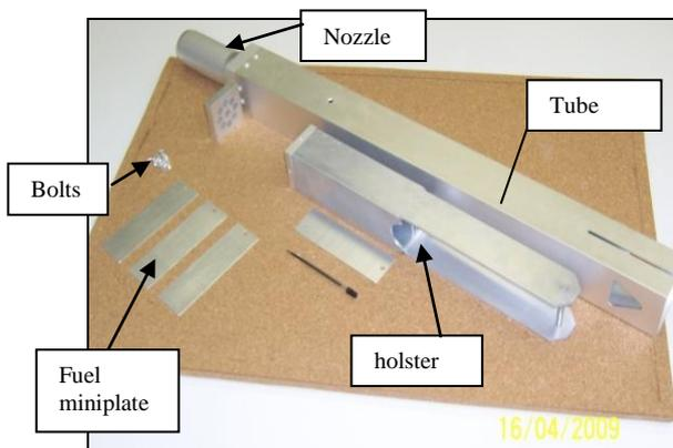
**Figure 1. Miniplate irradiation device (MID)**
