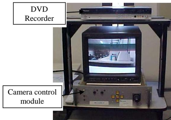
**Figure 3. Camera control module.**
