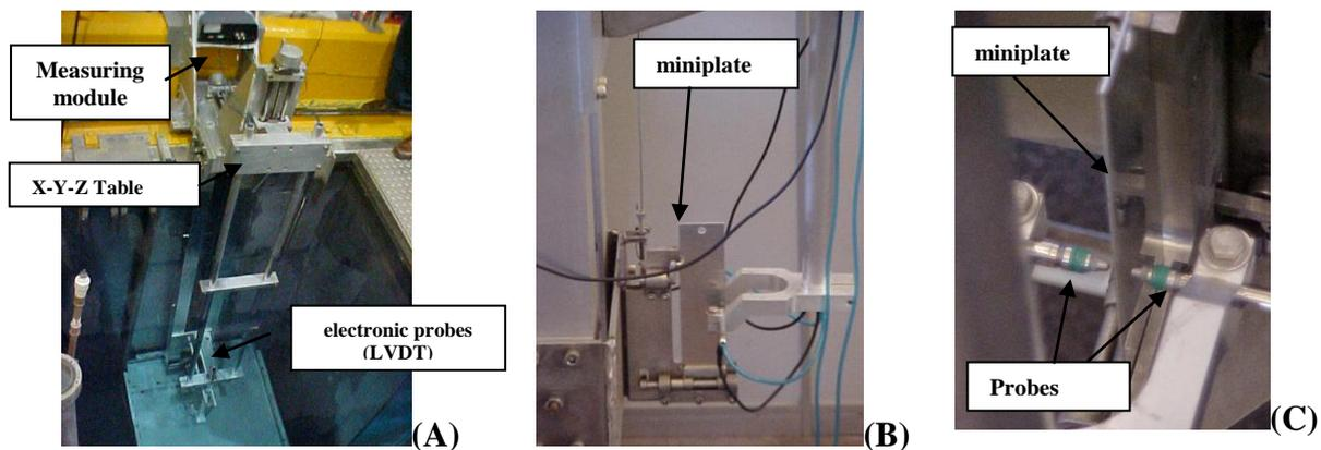
**Figure 5. FMTMS bench inside the IEA-R1 pool: (A) Structure of metal assembled on the edge of the pool; (B) e (C) Fuel miniplate at the measuring position.**
