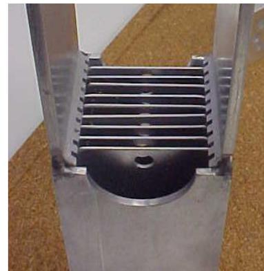
**Figure 2. Fuel miniplates assembled inside the holster.**
