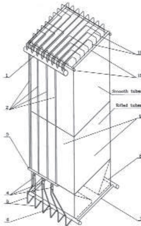
Figure 1. Scheme of the steam boiler evaporator
