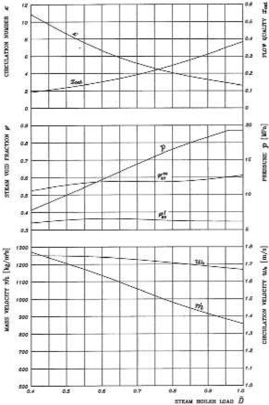
Figure 3. Calculated thermal-hydraulic parameters for the evaporator forced circulation.
