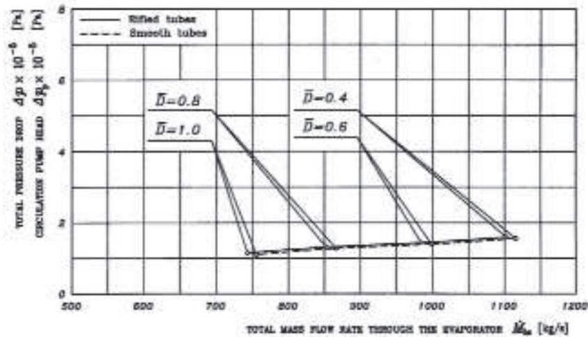
Figure 2. Hydraulic characteristic of the evaporator with the forced circulation in cases of rifled and smooth tubes.
