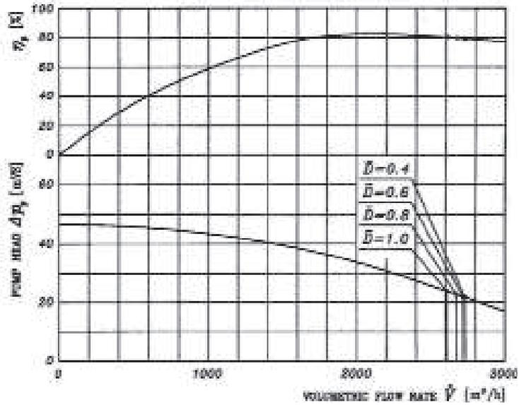
Figure 4. Evaporator operating points dependence on the boiler load
