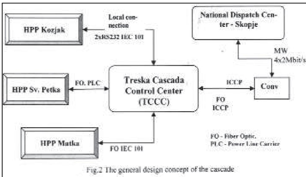
**Fig.2 The general design concept of the cascade**
