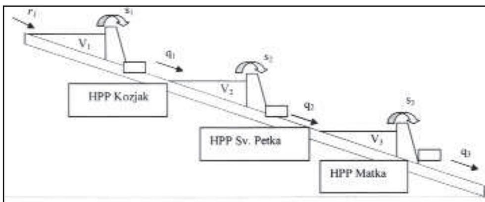
Fig.1 Hydraulically coupled hydroelectric plants in Treska Cascade
