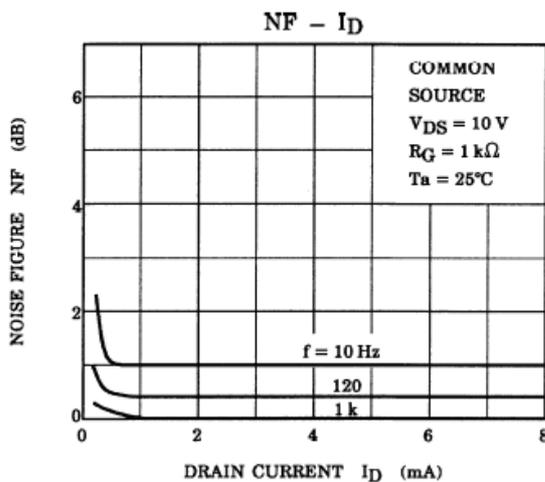
Fig. 3 – Noise figure for the 2SK170 transistor
