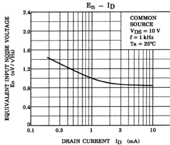
Fig. 5 – Equivalent input noise voltage for the 2SK170 transistor
