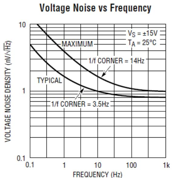
Fig. 6 – Voltage noise density versus frequency for the LT1028A op amp
