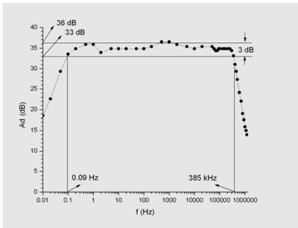
Fig. 7 – Amplifier voltage gain versus frequency
