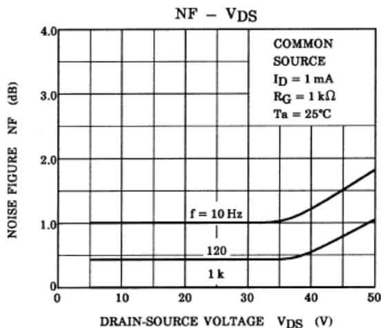
Fig. 4 – Noise figure for the 2SK170 transistor
