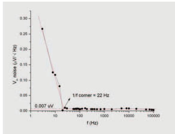
Fig. 8 – Equivalent input noise voltage of the amplifier versus frequency
