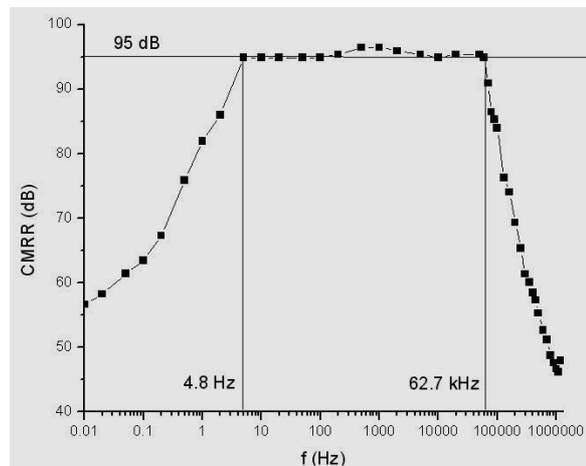
Fig. 9 – Common mode rejection ratio versus frequency
