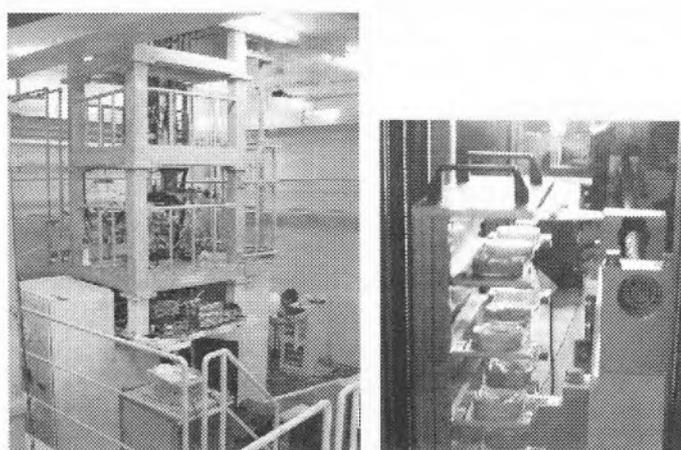
Figure 3. Irradiation with 320 MeV  $^{12}\text{C}^{6+}$  ions accelerated by AVF Cyclotron at TIARA (right), aluminium plates with petri dishes are inserted in the irradiation apparatus (left)
