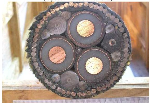
Figure 3: Cross section in three-core cable specimen (System 1- Scenario b).
