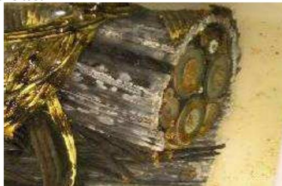
Figure 7: Final appearance of damaged three-core cable after leaching test.
