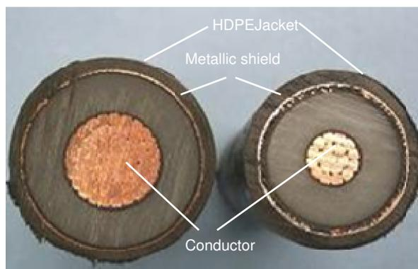
Figure 4: Cross section of the two single-core cables with aluminium sheet and copper wires (right) and with helicoidally copper tape (left).
