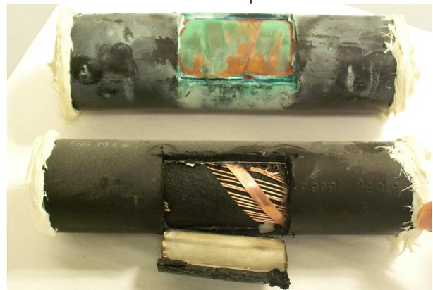
Figure 15: Final appearance of single-core cable with helicoidally copper tape (top) and single-core cable with aluminium sheet + copper wires (bottom).
