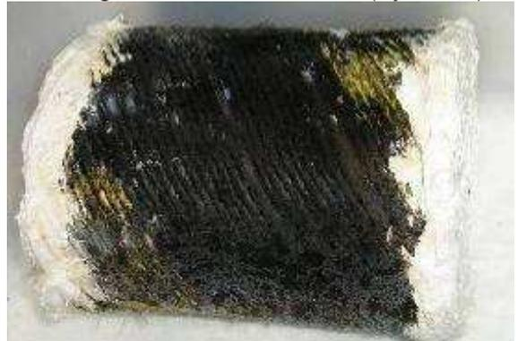
Figure 2: Sealed three-core cable specimen (System 1-Scenario a).
