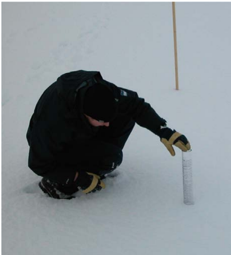
Figure 4-1. Measurement of snow depth with plastic tube at Storskäret, AFM000071.
