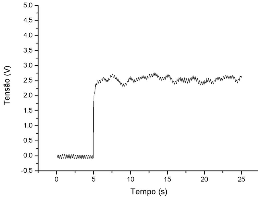
**Figure 3 – A typical in-plant LCSR test.**
