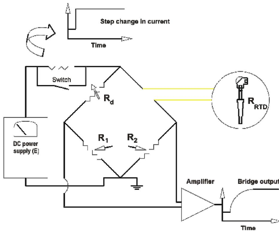
Figure 2 - Wheatstone bridge used in RTDs LCSR tests.
