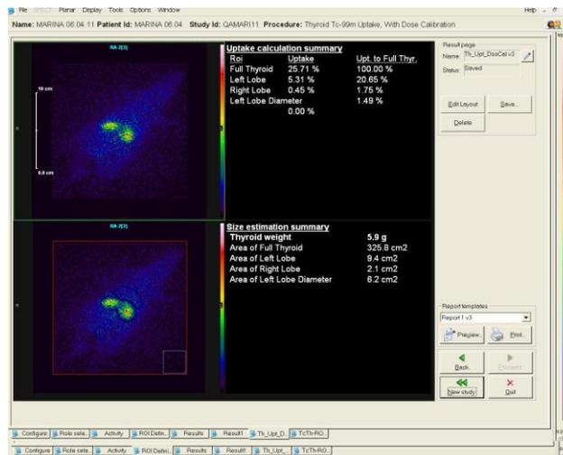
**Figure 1. Gamma camera ROI tools to calculate the concentration of activity (Rat A). The equipment parameters fixed to <sup>99m</sup>Tc studies, would be interpreted as: full thyroid (whole body), left lobe (kidneys), right lobe (liver) and left lobe diameter (urinary bladder).**
