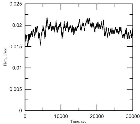
**Figure 13. Excursion of the natural circulation flow in hot leg.**
