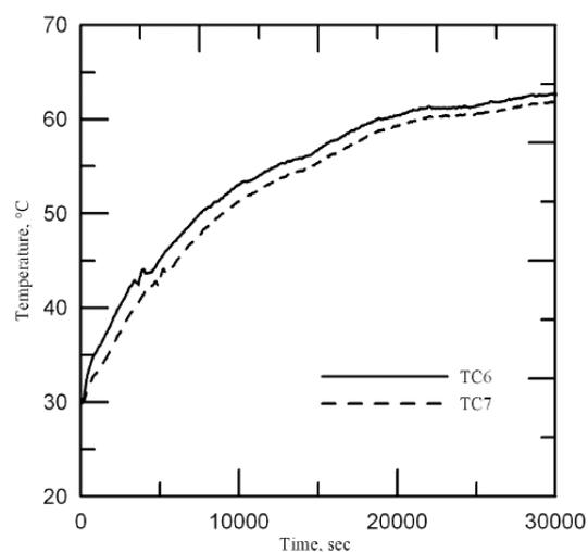
**Figure 10. Temperatures in heat exchanger, fluid and tube wall.**
