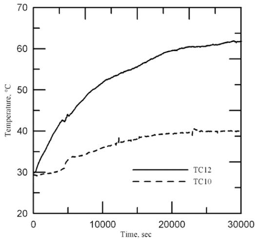
**Figure 7. Input and output of secondary cooling system.**
