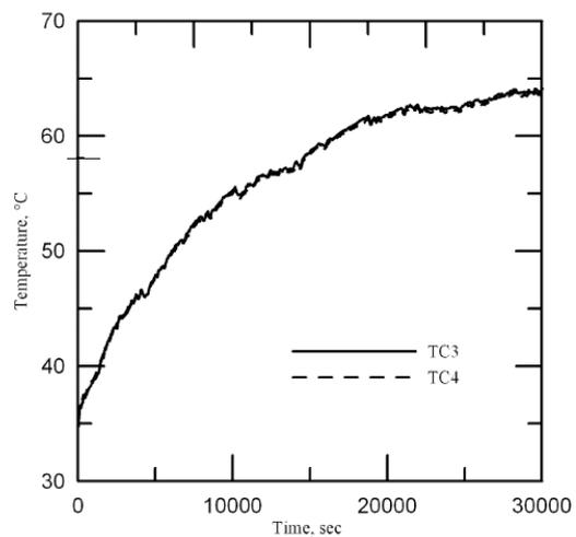
**Figure 6. Temperatures in the medium point of hot leg and heater output.**
