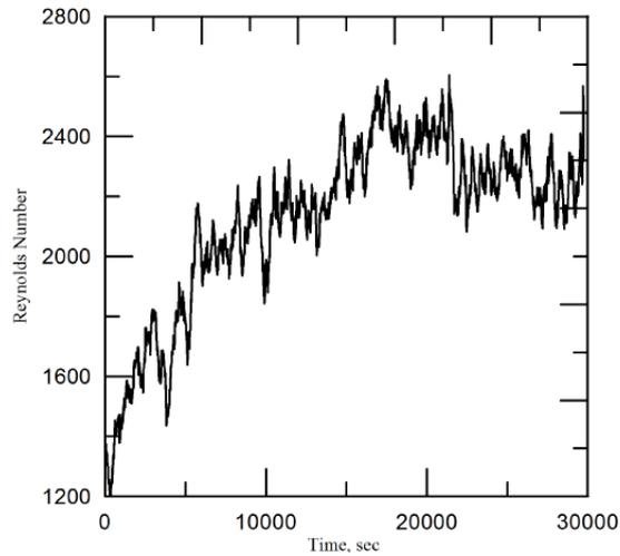
**Figure 14. Reynolds number in hot leg tube.**
