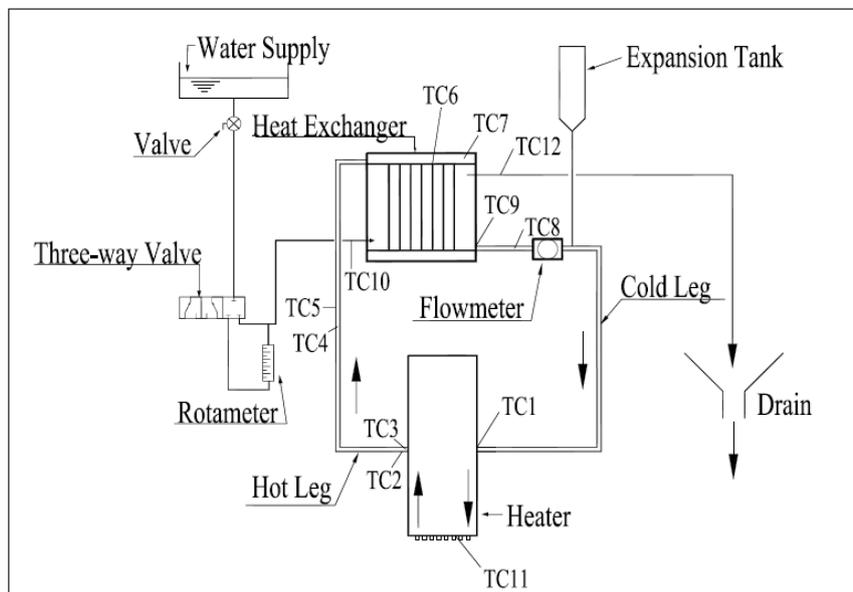
**Figure 2. Schematic of natural circulation circuit and points of measurements through thermocouples.**
