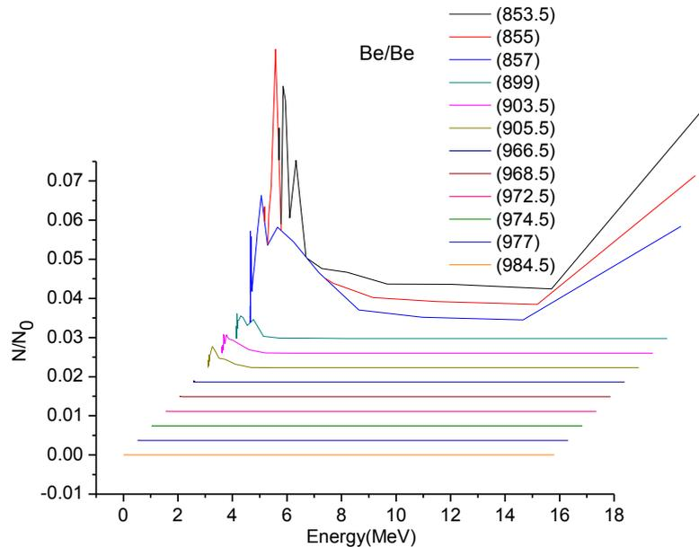
**Figure 4 - Neutron spectrum for Be-Be coating.**
