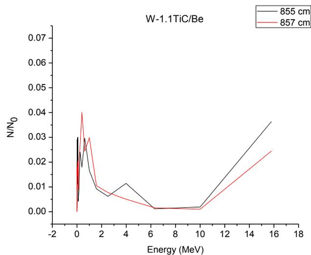
**Figure 11. Neutron Fluence at 857cm from the centre in the shield block.**
