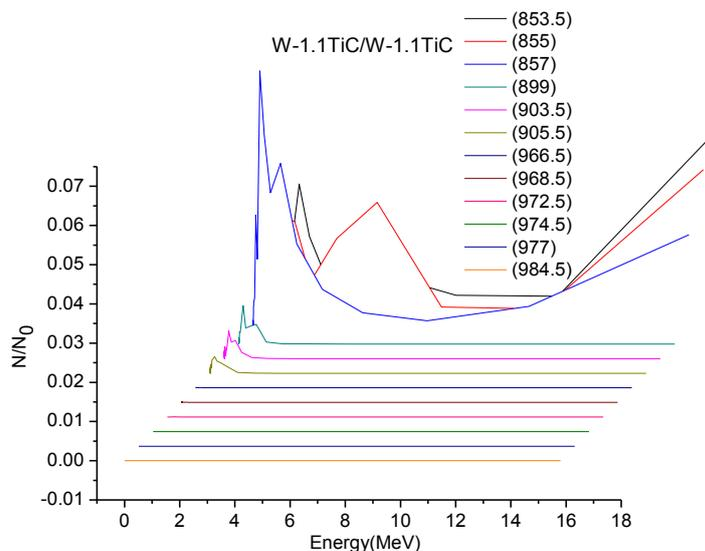
**Figure 5. Neutron spectrum for W1.1TiC/W1.1TiC coating.**
