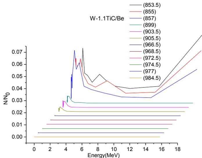
**Figure 6. Neutron fluence results for W-Be arrangement.**
