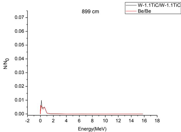
**Figure 9. Neutron fluence at 899 cm from the centre.**
