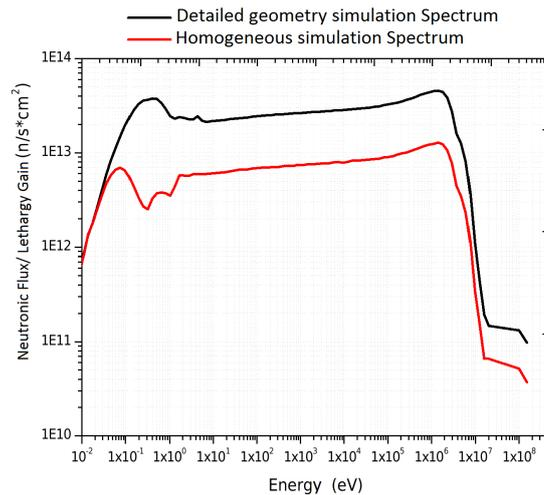
Figure 15: Comparison between the energetic spectrum obtained using an homogeneous and heterogeneous simulation of the TRISO particles
