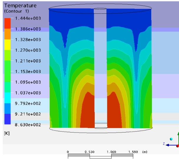
Figure 10: Axial-radial temperature profile.
