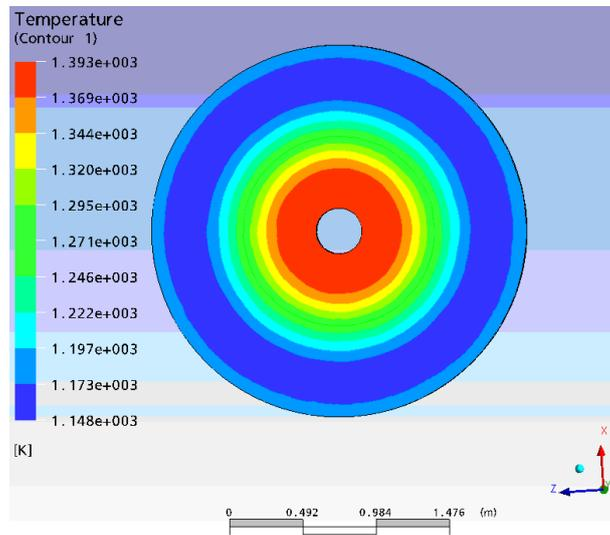
Figure 13: Outlet temperature profile corresponding to the axial-radial power density distribution.
