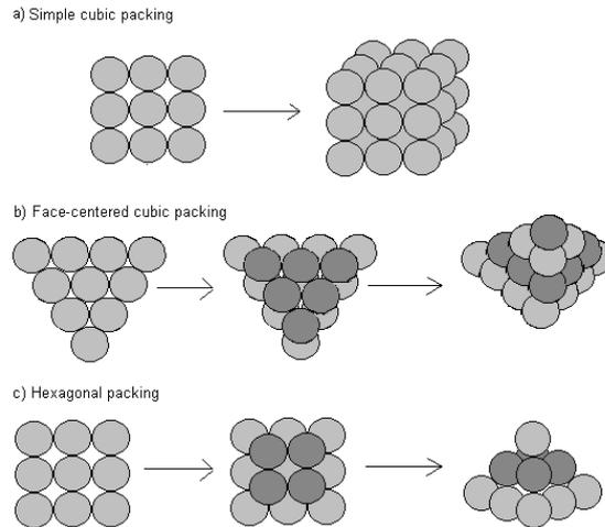
Figure 2: Three dimensional arrangements for identical balls.
