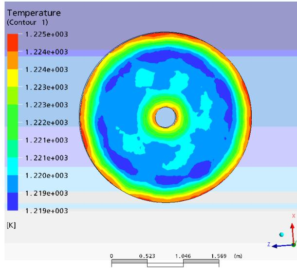
Figure 11: Outlet temperature profile corresponding to the axial power density distribution.
