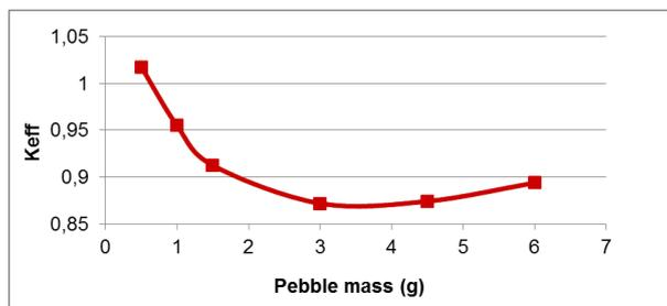
Figure 5:  $K_{eff}$  vs. fuel mass per pebble.
