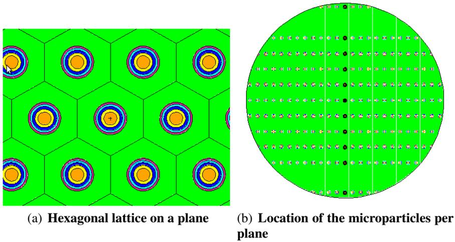
Figure 14: Distribution of TRISO particles inside the pebble
