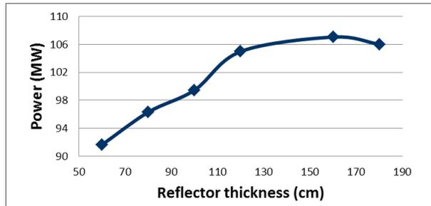
Figure 4: Total power vs. radial reflector thickness for the EOC.
