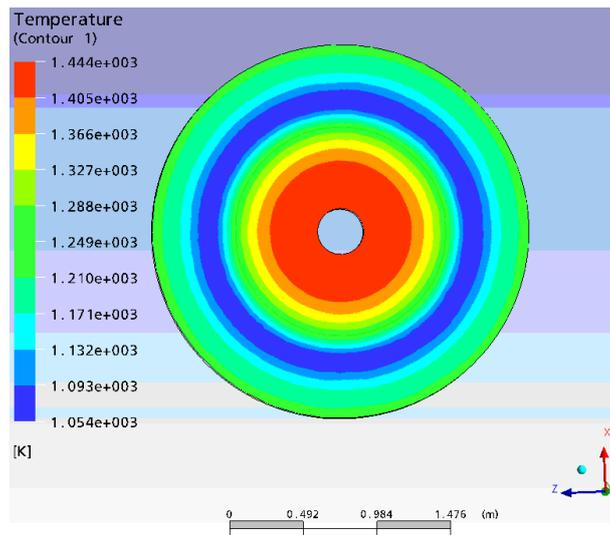
Figure 12: Outlet temperature profile corresponding to the radial power density distribution.
