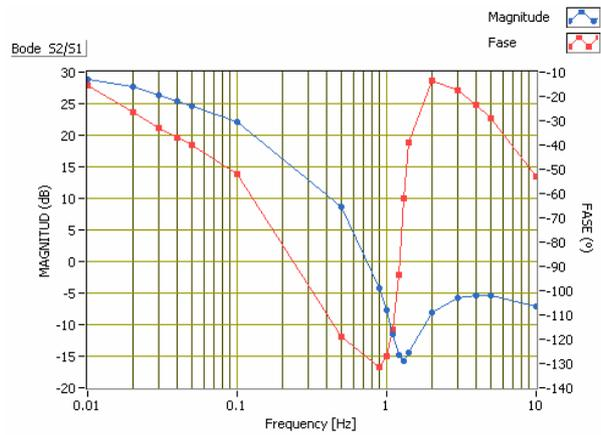
**Figure 8. Bode diagram Pressure signal vs. C85**
