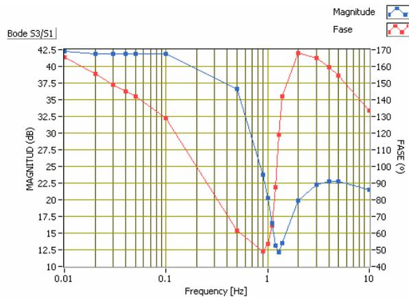
**Figure 9. Bode diagram Pressure signal vs. N32**
