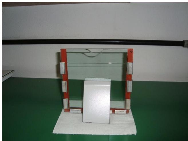
**Figure 2. Sample holder for the flat solid source.**
