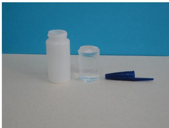
**Figure 1. The plastic container and the cylindrical acrylamide polymerized resin.**
