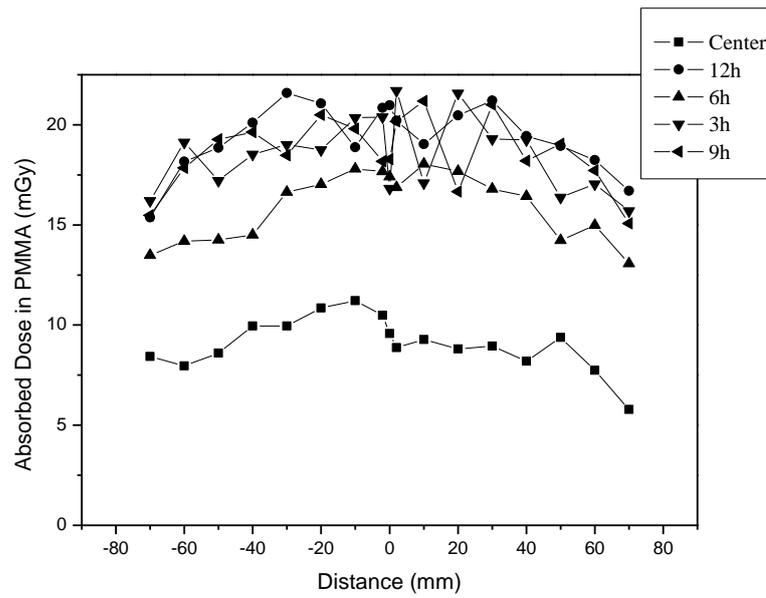
**Figure 4. Dose variation of SI along the longitudinal axis of five positions in the PMMA phantom.**
