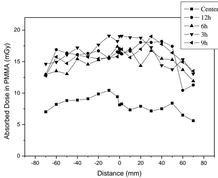
**Figure 6. Dose variation of SIII along the longitudinal axis of five positions in the PMMA phantom.**
