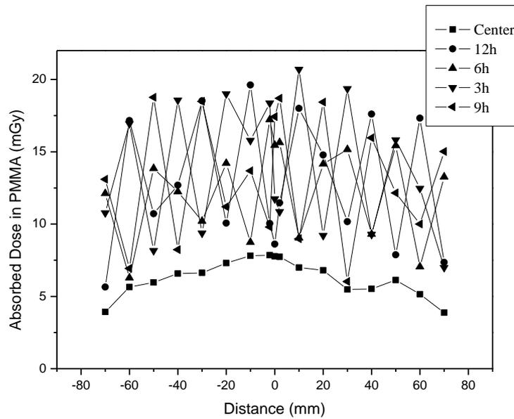
**Figure 7. Dose variation of SIV along the longitudinal axis of five positions in the PMMA phantom.**
