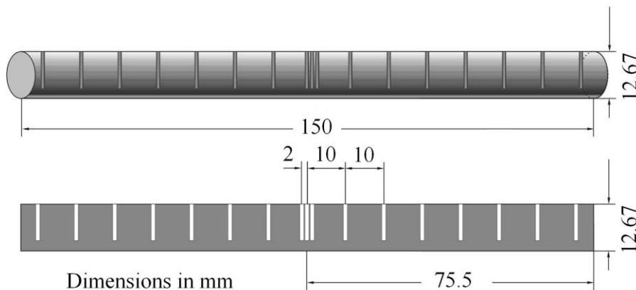
**Figure 2. PMMA cylinder for positioning the TL dosimeters.**
