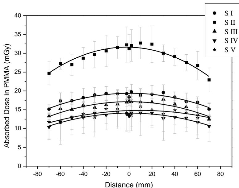
**Figure 9. Comparison of the variation of the average doses in the longitudinal axis of the peripheral cylinders in the five CT scanners studied.**
