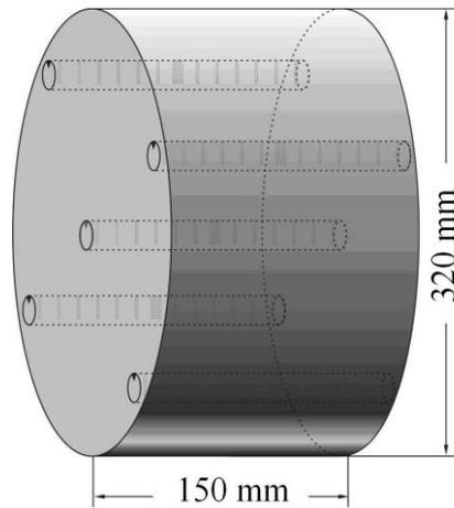
**Figure 1. Body PMMA phantom for CT dosimetry.**
