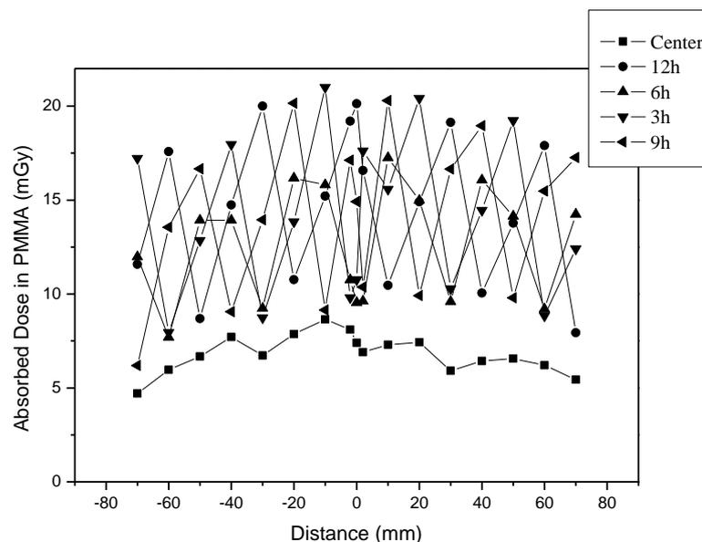
**Figure 8. Dose variation of SV along the longitudinal axis of five positions in the PMMA phantom.**
