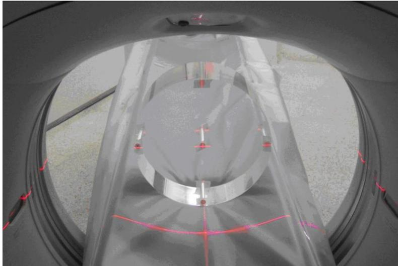
**Figure 3. Positioning of the PMMA phantom in the scanner isocenter.**
