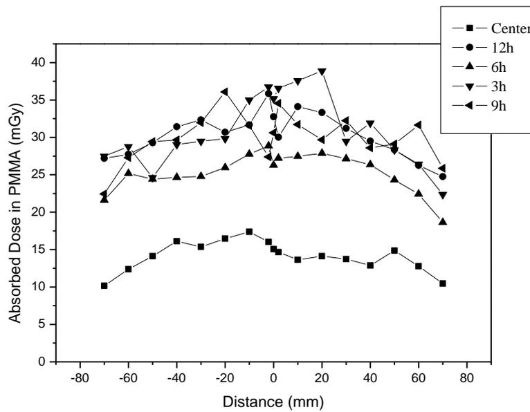
**Figure 5. Dose variation of SII along the longitudinal axis of five positions in the PMMA phantom.**
