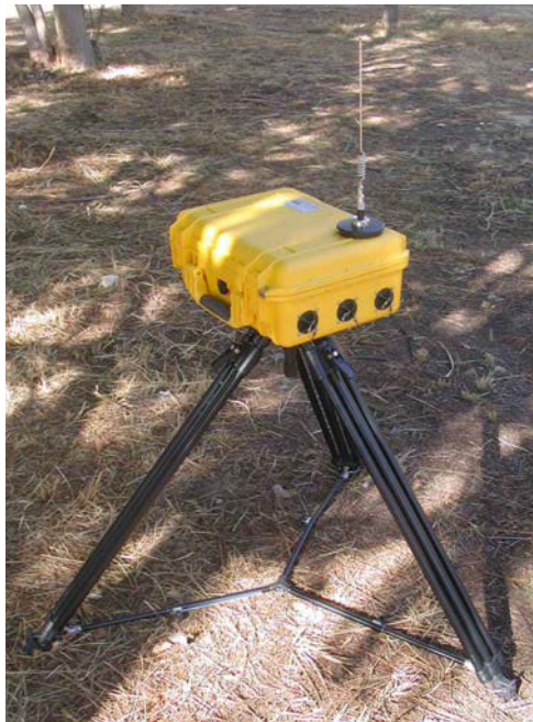
Figure 1: Deployed Radiation Monitoring Station
