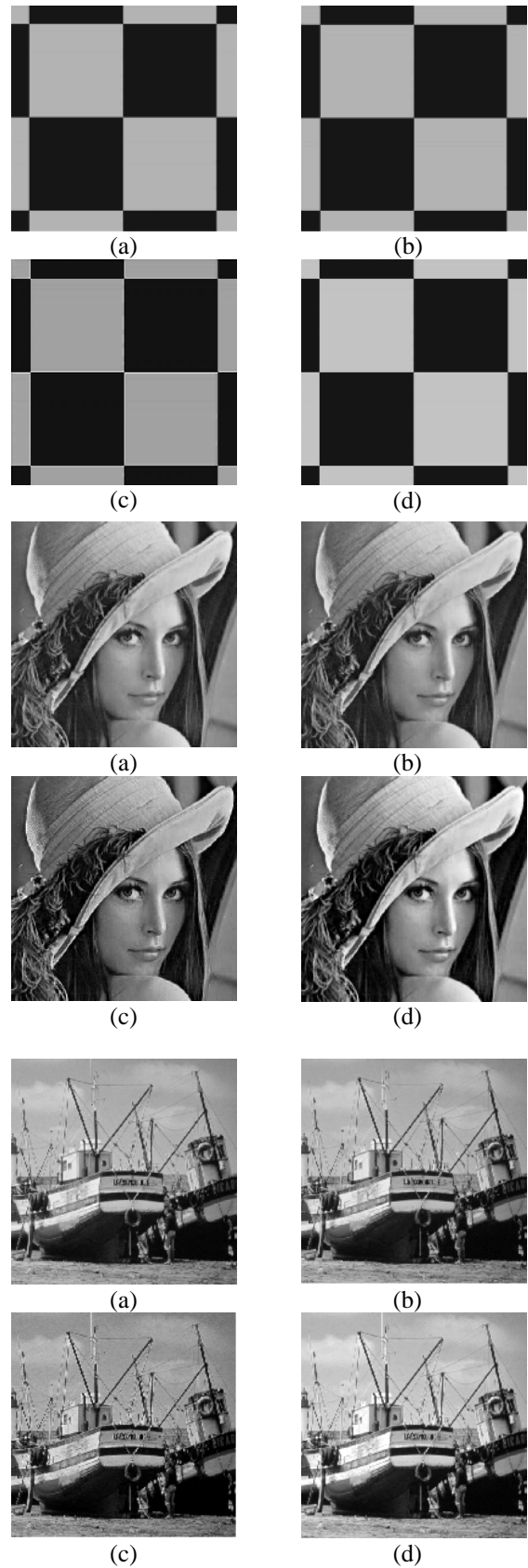
Figure 4. Result of contrast image Enhancement using different approaches, (a) original images, (b) Enhanced results using weighted median filter ( L = 0 and T = 15 ), (c) conventional unsharp masking method with k = 0.002 and (d) the proposed approach
