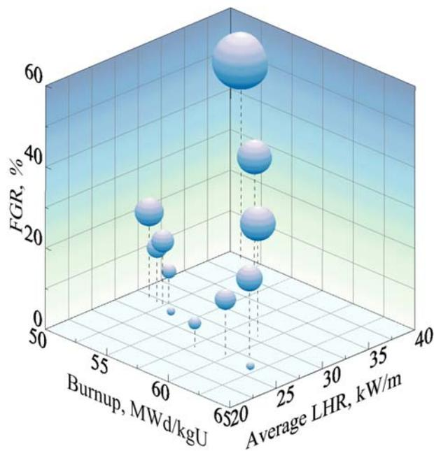
Figure 15. FGR in ~ 51...63 MWd/kgU burnup VVER fuel rods vs. ALHR (max value) under power cycling
