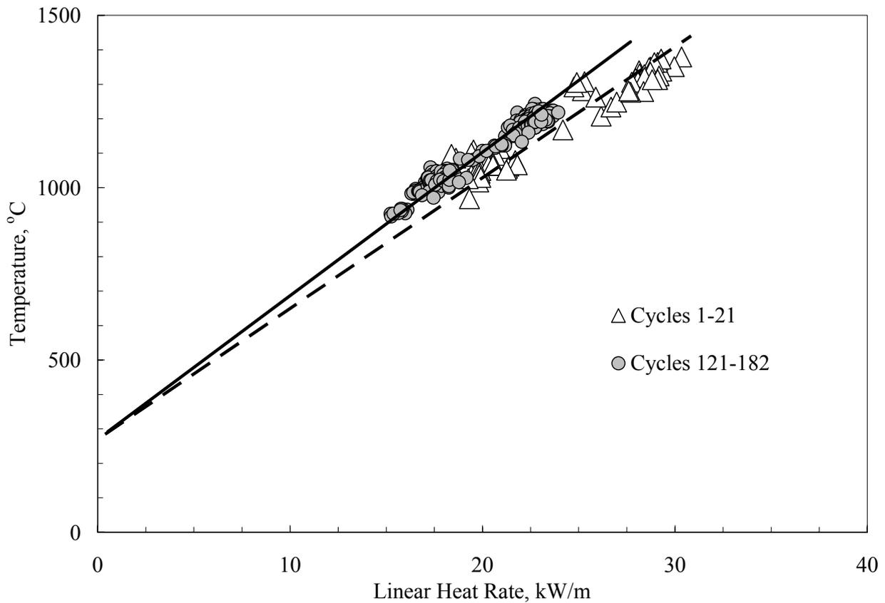
Figure 11. Fuel temperature vs. LHR at the place of thermocouple location for a  $\sim 50$  MWd/kgU burnup refabricated VVER-1000 fuel rod under power cycling for test parameters at a coolant temperature higher than  $255^{\circ}\text{C}$
