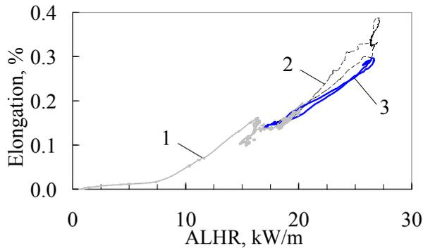
Figure 3. Relative elongation of  $\sim 51$  MWd/kgU
