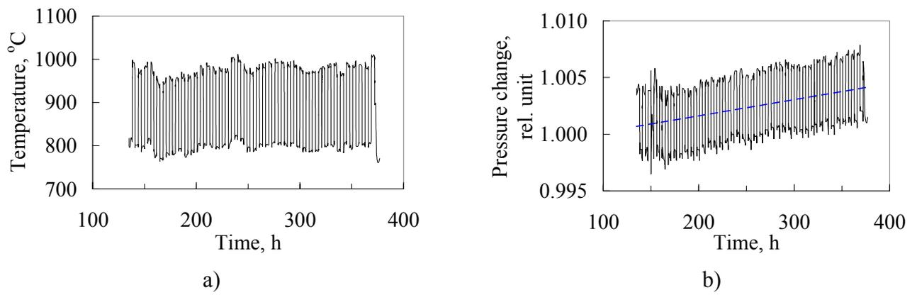
Figure 14. Change of fuel temperature (a) and under-cladding gas pressure (b) in the ~ 49 MWd/kgU burnup refabricated VVER-1000 fuel rod under power cycling (cycles 1-40)
