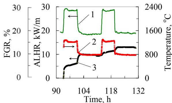
Figure 13. Change of ALHR (1), fuel temperature (2) and FGR (3) for  $\sim 51$  MWd/kgU burnup refabricated VVER-440 fuel rod under power cycling
