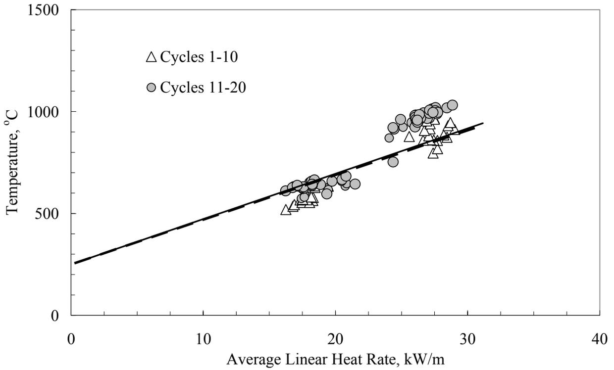
Figure 9. Fuel temperature vs. ALHR for a ~ 60 MWd/kgU burnup refabricated VVER-440 fuel rod under power cycling
