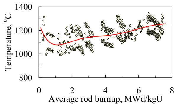
Figure 12. Change in the  $\sim 50$  MWd/kgU burnup refabricated VVER-1000 fuel rod temperature normalized to the LHR equal to  $22$  kW/m at the thermocouple location vs. the average fuel rod burnup increment under power cycling
