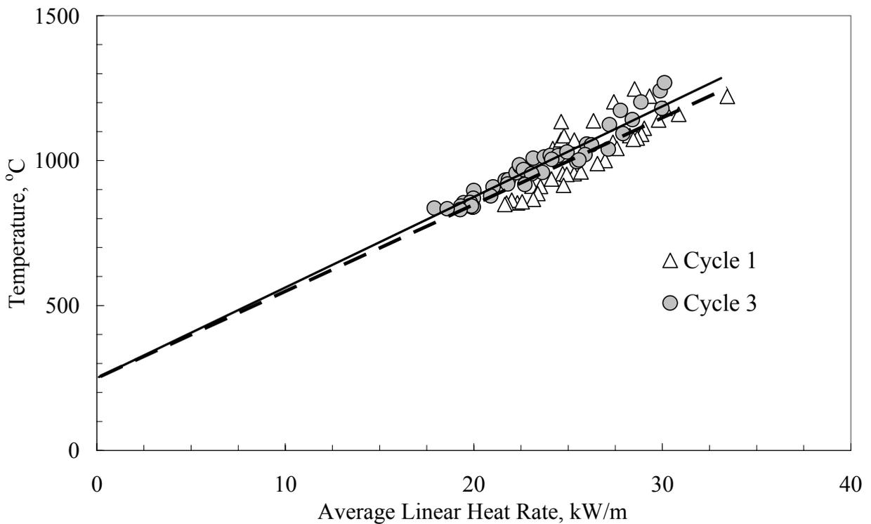
Figure 8. Fuel temperature vs. ALHR for a  $\sim 51$  MWd/kgU burnup refabricated VVER-440 fuel rod under power cycling
