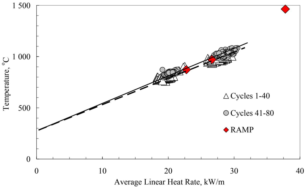
Figure 10. Fuel temperature vs. ALHR for a ~ 49 MWd/kgU burnup refabricated VVER-1000 fuel rod under power cycling
