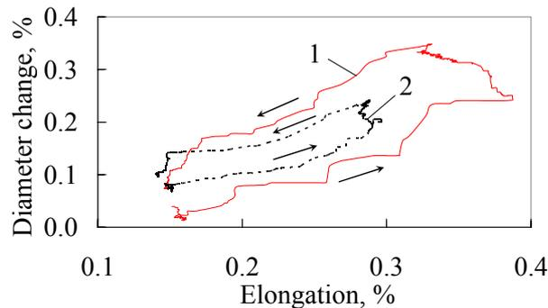
Figure 5. Relative elongation vs. relative diameter change of  $\sim 51$  MWd/kgU burnup
