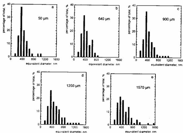
Fig. 8. Sub-grain size histograms for various depth from fuel surface [19].
