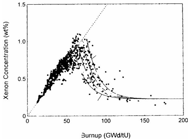
Fig. 5. Local xenon concentration as a function of the local burn-up; the threshold burnup was varied between 60 and 75 GWD/tU.[14]
