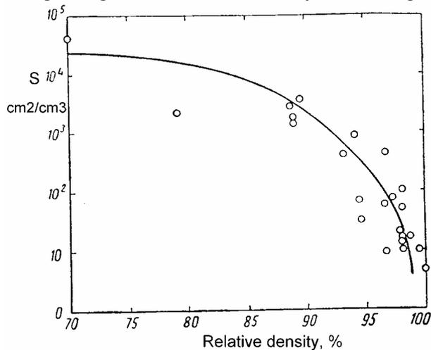
Fig. 1. Total surface area  $S$  [ $\text{cm}^2/\text{cm}^3$ ] versus relative density [%] of sintered  $\text{UO}_2$  [1].
