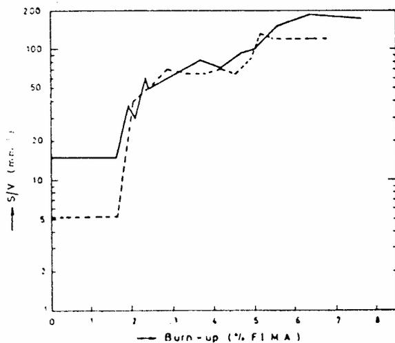
Fig. 3. ( $S/V$ ) plotted against burn-up for two different specimens [12].
