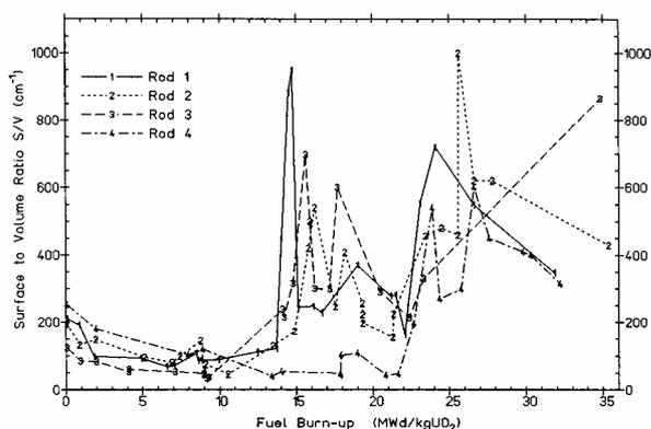
Fig. 4. Surface to volume ratio plotted as a function of burn-up [13]
