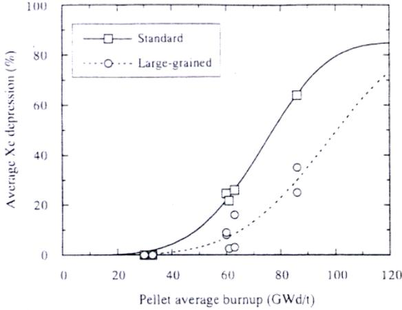
Fig. 7. Burnup dependence of average Xe depression in pellet outside region for fuel pellets irradiated in IFA551 and IFA566 rigs [16].
