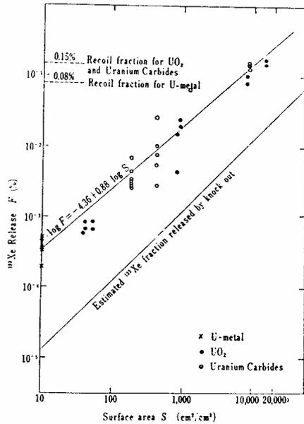
Fig. 2. The fraction of  $^{133}\text{Xe}$  released the void space of the capsule [4].
