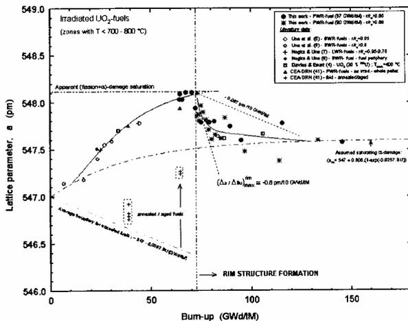
Fig. 8. Lattice parameter of irradiated fuels versus local burn-up ( $T < 800^\circ C$ ) [17].
