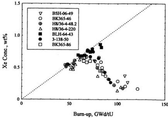
Fig. 6. Local concentration of xenon measured by EPMA in the outer region of the fuel [15].
