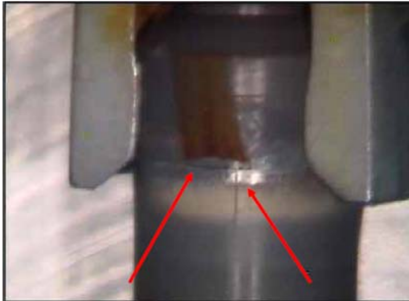
Fig. 4 An example of the upper weld leaker
