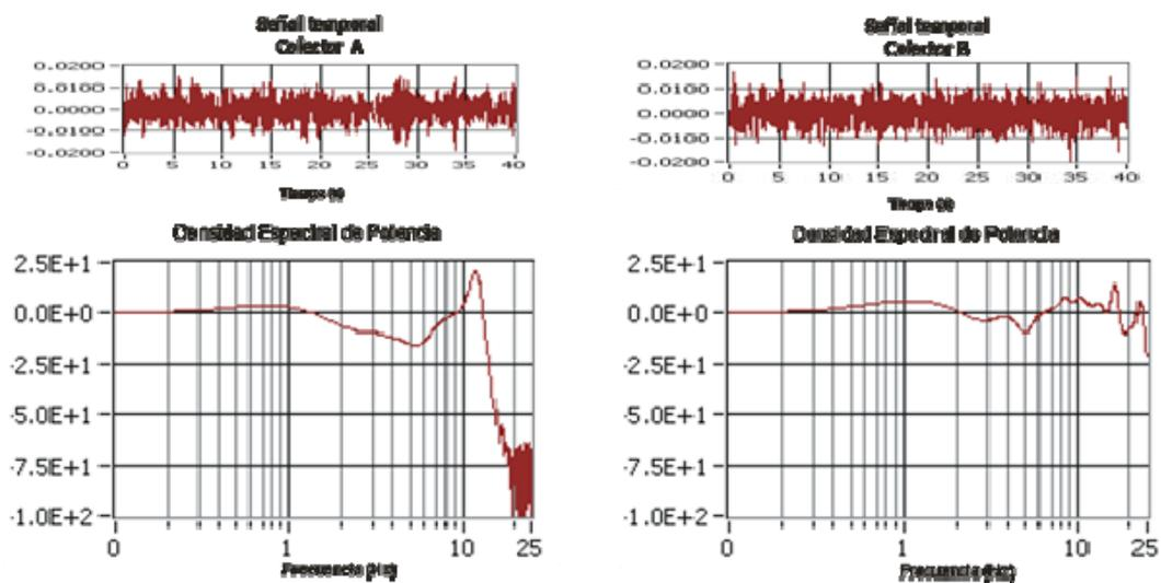
Figure 6. Analysis of redundant instrumentation signals (Sensors A and B)
