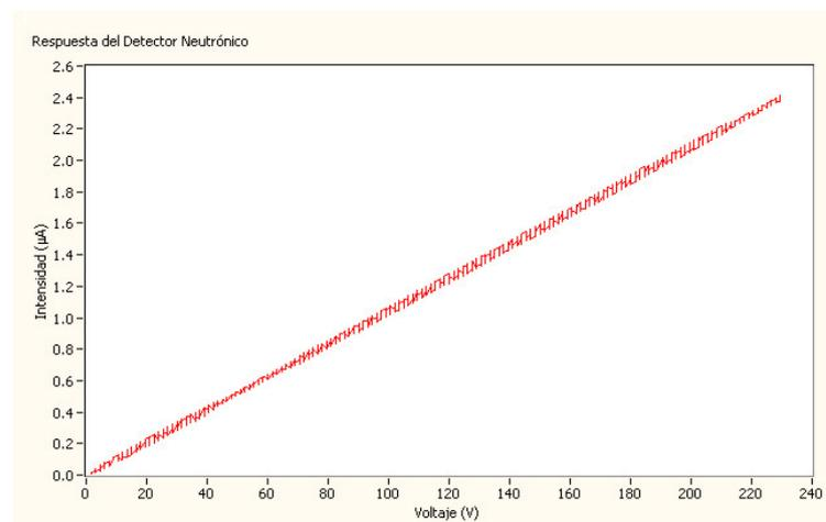
**Figure 11: LPRM response in operation with a malfunction.**
