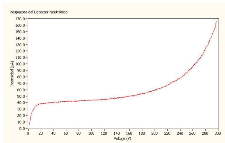
**Figure 10: LPRM response reference in operation.**
