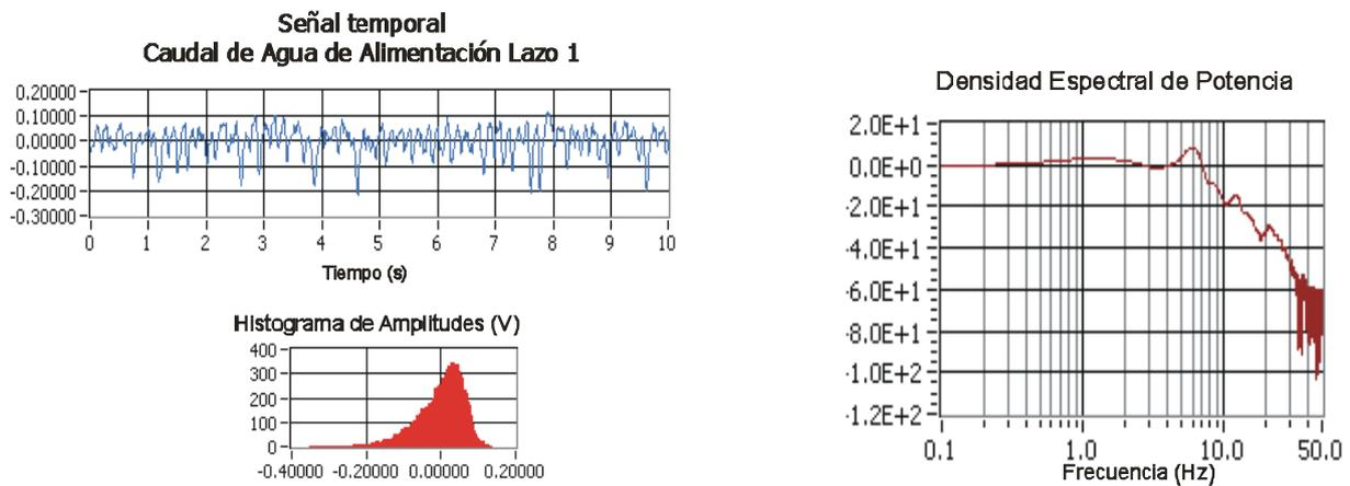
**Figure 3. Air presence in feed water lines.**
