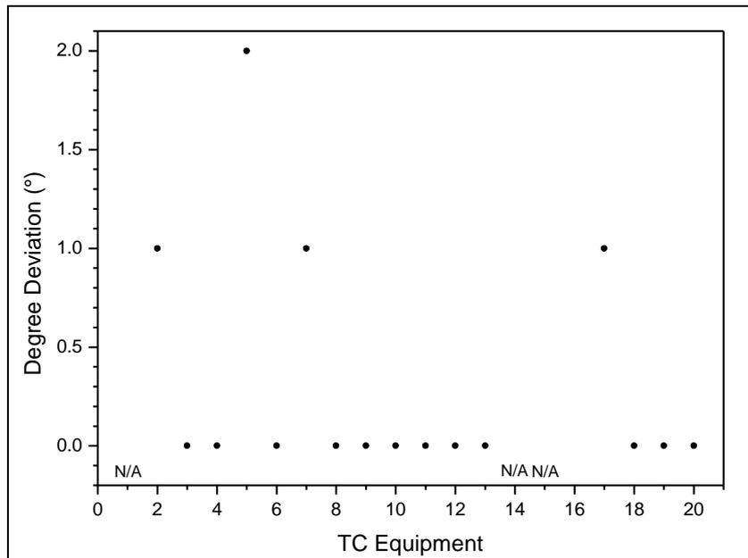
Figure 4 – Assessment of gantry tilt accuracy.
