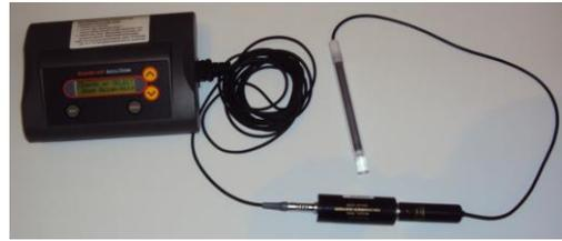
Figure 2 – CT ionization chamber.
