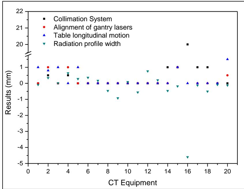
Figure 3 – Assessment of collimation system, alignment of gantry lasers with the center of imaging plane, table longitudinal motion and radiation profile width.
