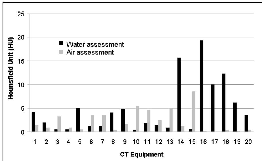
Figure 6 – Accuracy of the CT number in water and air assessment.
