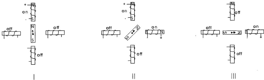
Figure 1: Control rod controller movement
