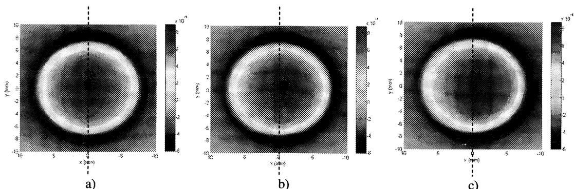
Figure 2: Simulated differential magnetic field visualization at 1ms for (a) 0° angular defect (b) 20° angular defect (c) 40° angular defect
