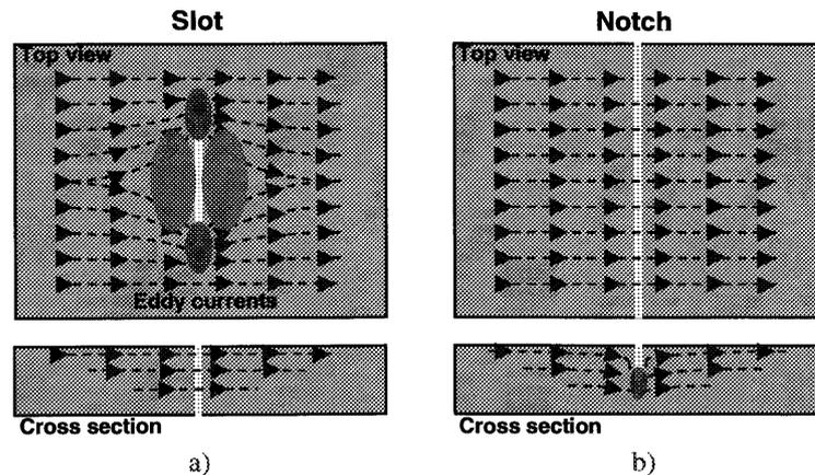
Figure 5: Theoretical (a) eddy current and b) heat distribution for ideal slot and notch
