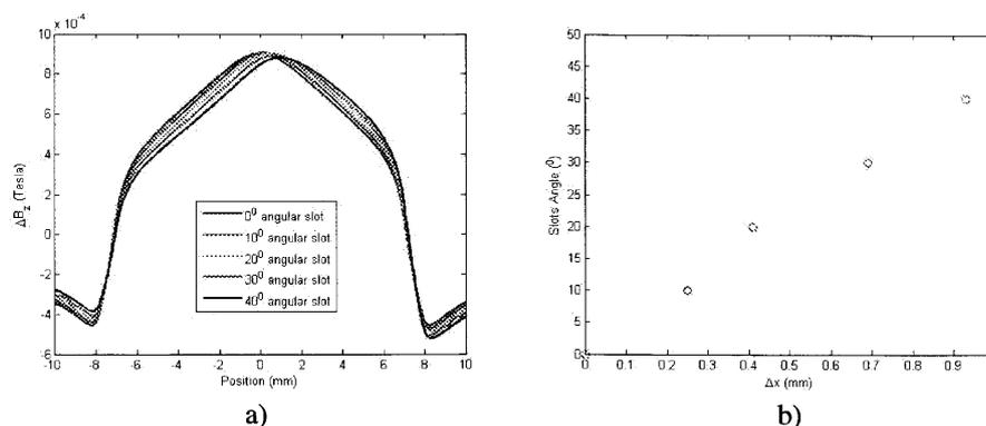
Figure 3: (a) Differential magnetic field distribution against angular defect (b) Correlation between peak distribution shift and defect angle
