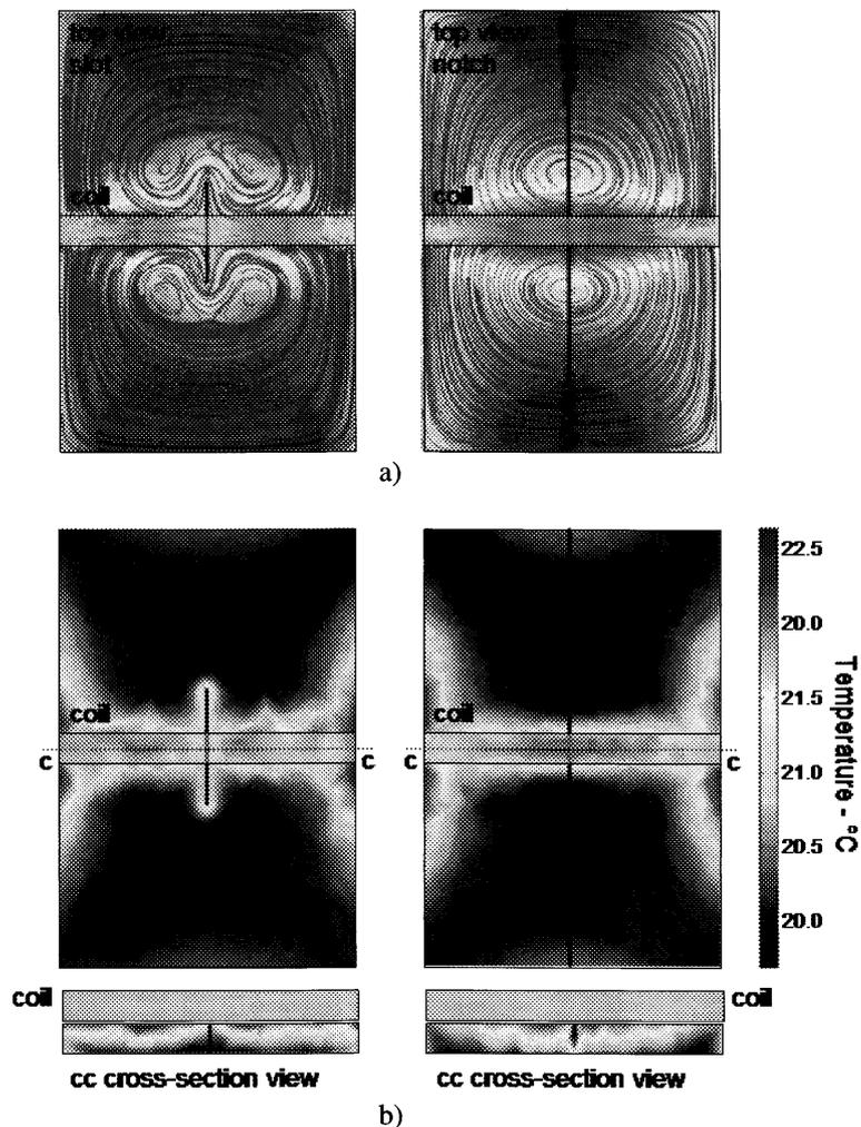
Figure 4: Simulation results of (a) eddy current and (b) heat distribution for ideal slot and notch
