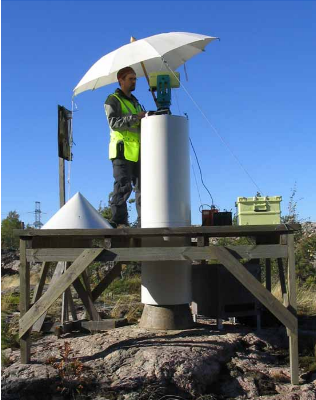
Figure 5-1. The mekometer Kern ME5000 at the pillar GPS8 during baseline observation on October 2005. (Photograph T. Ahola 2005.)
