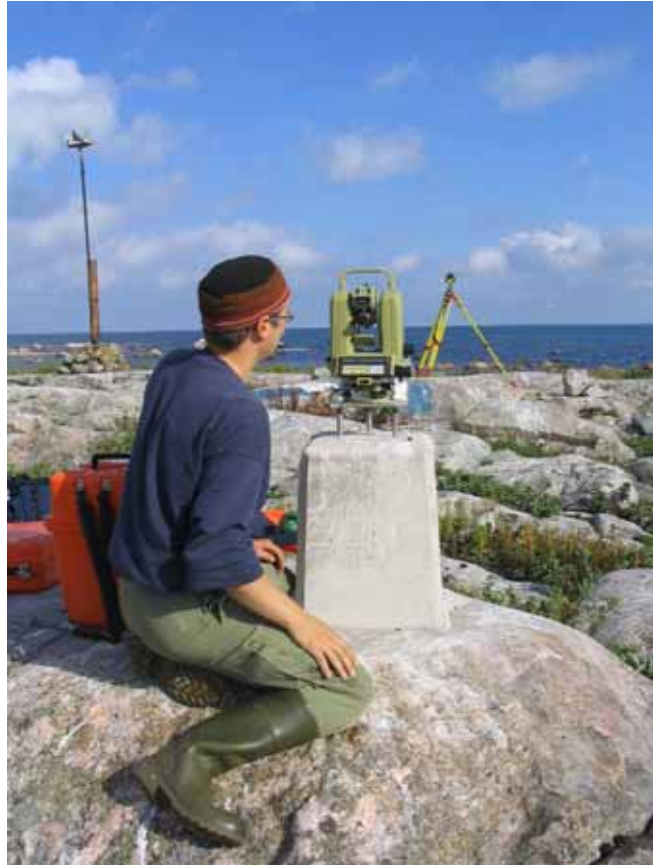
Figure 6-1. The distances between pillars and reserve markers were measured using the Distomat Wild DI2002 EDM instrument. The horizontal and vertical angles were observed with the theodolite Theomat Wild T2002. (Photograph T. Ahola 2005.)
