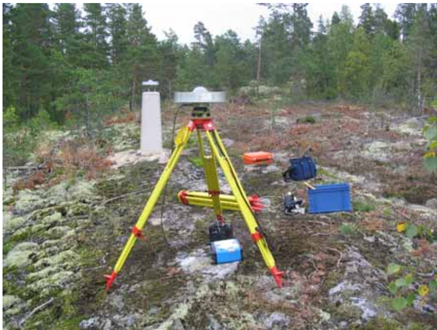
Figure 6-2. The determinations of the azimuths have been made using GPS observations. (Photograph J. Ahola 2004.)
