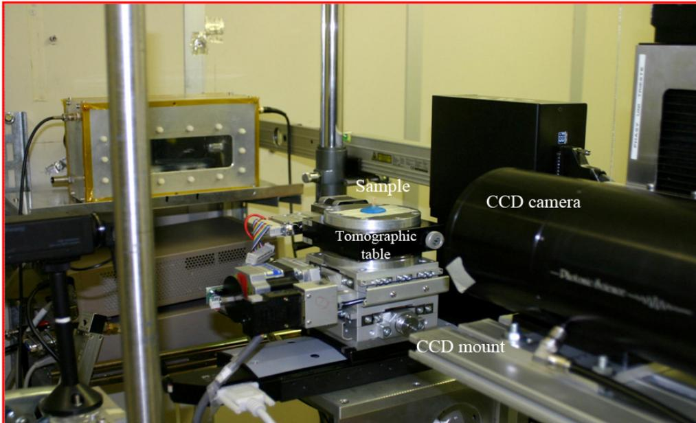
**Figure 1. Microcomputed tomography system at SYRMEP beamline**
