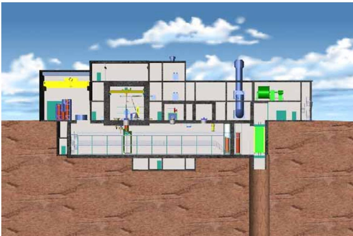
**Figure 6.** Longitudinal section of the encapsulation plant. On lowest level: Canister transfer corridor and canister loading area. On ground level from left to right: Spent fuel cask reception and storage area for empty canisters, fuel handling cell and repair shop above the handling cell. In the middle: welding chamber. To the right: inspection chamber and ventilation equipment room for the repository's controlled area.
