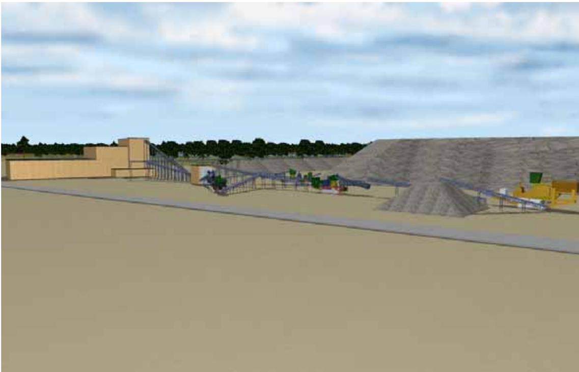
*Figure 16. Broken rock storage on the right, crusher station in the center and crushed rock storage in the background. The backfill material mixing station is on the left in the figure.*
