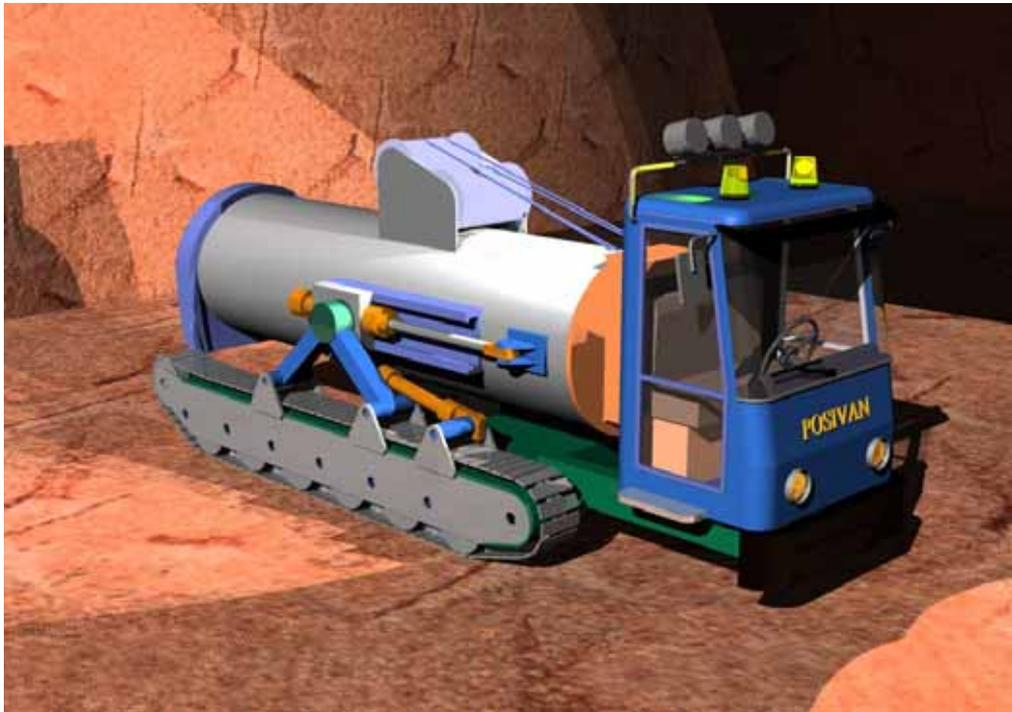
*Figure 7. Canister transfer and installation vehicle.*
