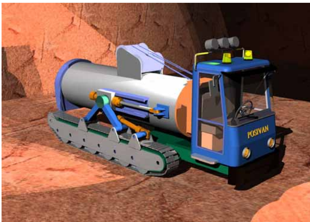
Figure 9. Canister transfer and installation vehicle.
