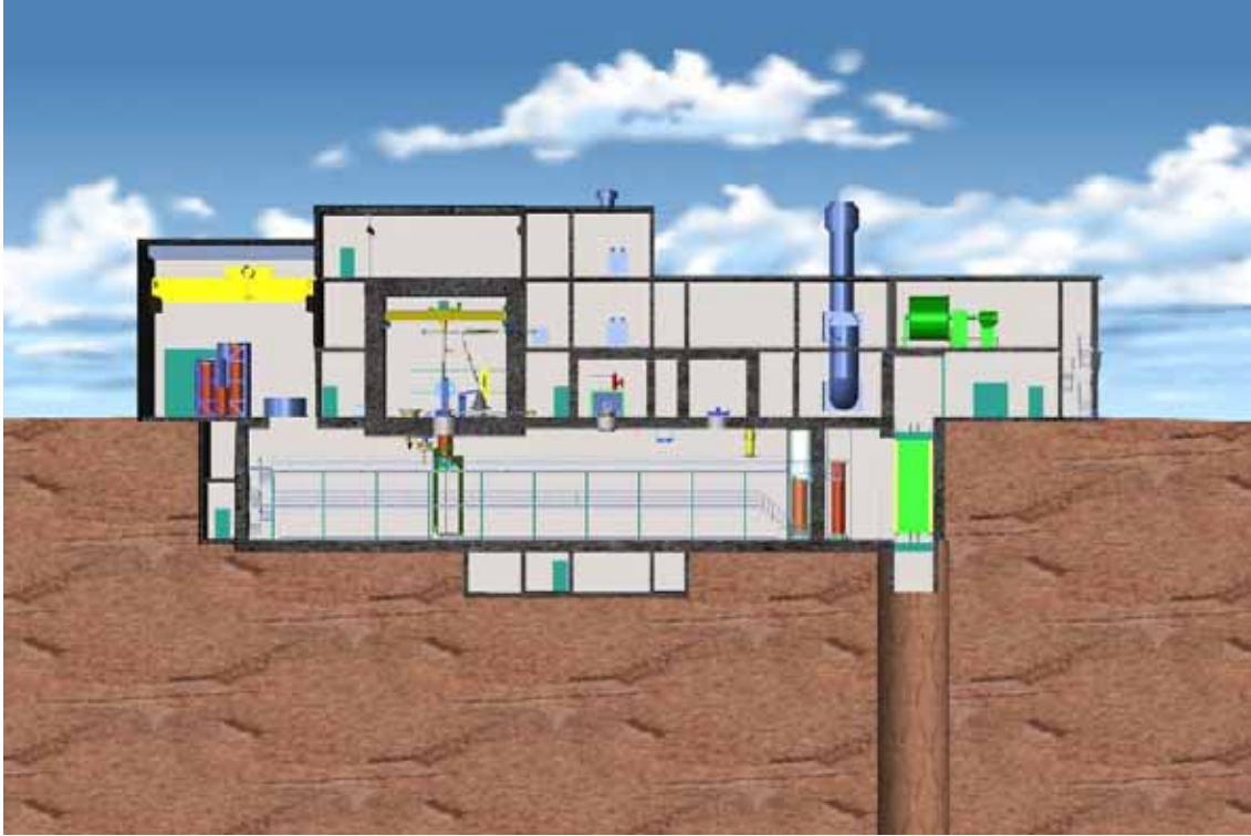
Figure 7. Longitudinal section of the encapsulation plant. On lowest level: Canister transfer corridor and canister shaft. On ground level from left to right: Spent fuel cask reception and storage area for empty canisters, fuel handling cell and repair shop above the handling cell. In the middle: welding chamber. To the right: inspection chamber and ventilation equipment room for the repository's controlled area.
