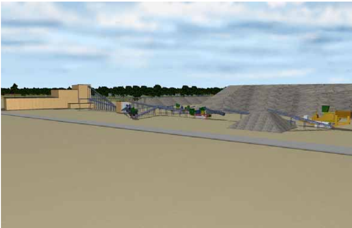
Figure 17. Broken rock storage on the right, crusher station in the center and crushed rock storage in the background. The backfill material mixing station is on the left in the figure.
