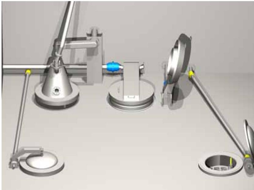
**Figure 1.** A view of the handling cell. Drying chambers are visible on the sides and the spent fuel canister docking station, the protective cone, and the atmosphere changing cap furthest in the back.
