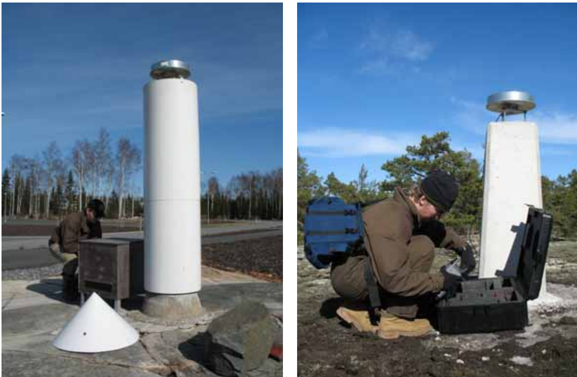
Figure 3-1. Left: The original GPS pillars are two meter high concrete platforms, which have metal layers for solar radiation. Right: New observation pillars are smaller than original ones. They have been established at the observation sites, but the original pillars have been made in a factory and then those pillars have been carried to the observation sites. (Photographs J. Ahola 2007.)
