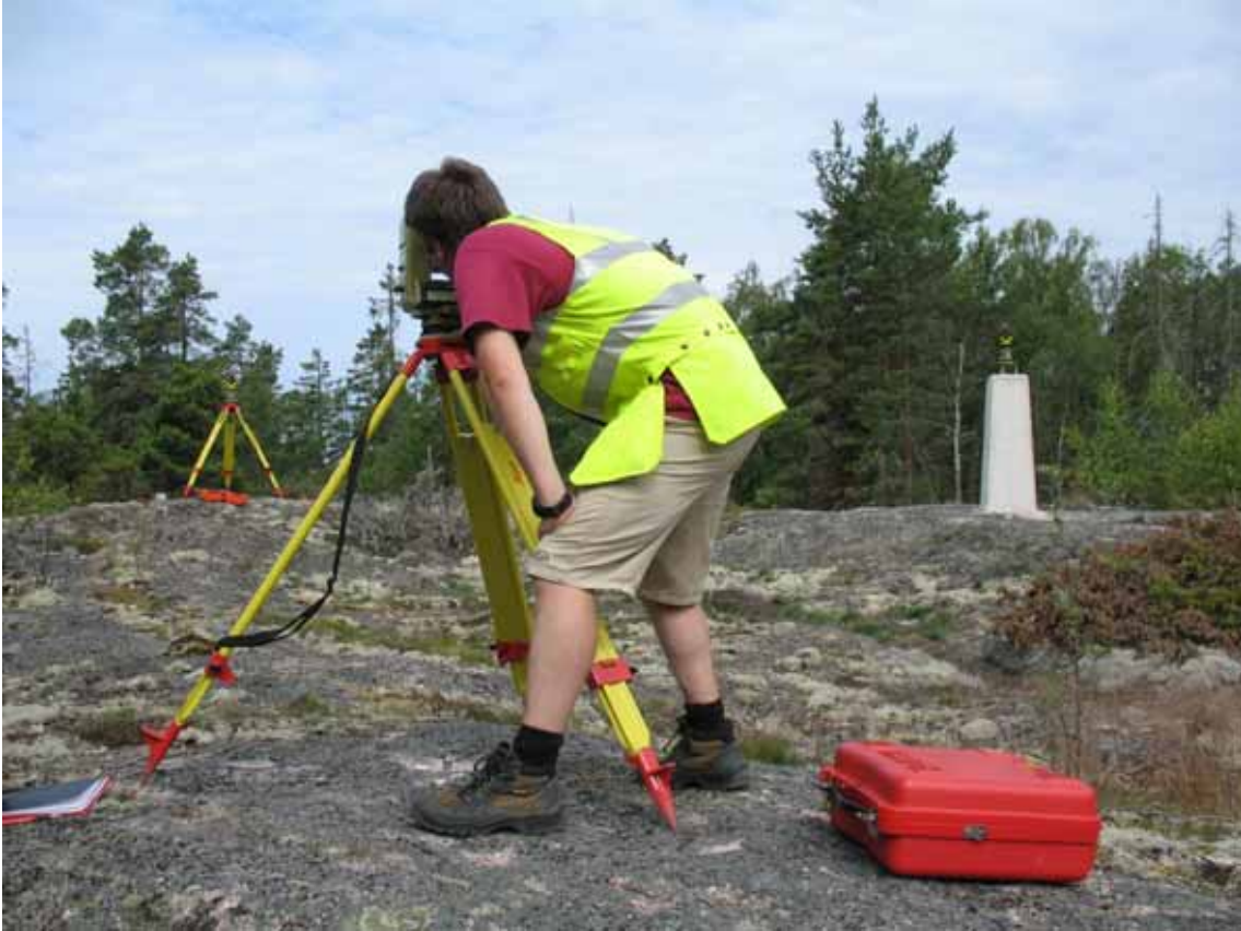
Figure 6-1. The distances between pillars and control markers were measured using the Distomat Wild DI2002 EDM instrument. The horizontal and vertical angles were observed with the theodolite Theomat Wild T2002. (Photograph T. Ahola 2007.)
