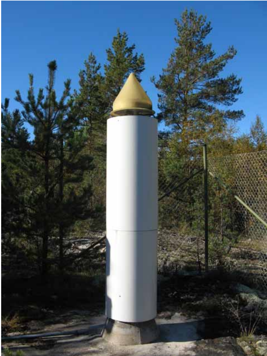
Figure 2-1. The permanent GPS station at Olkiluoto. (Photograph H. Koivula 2007.)
