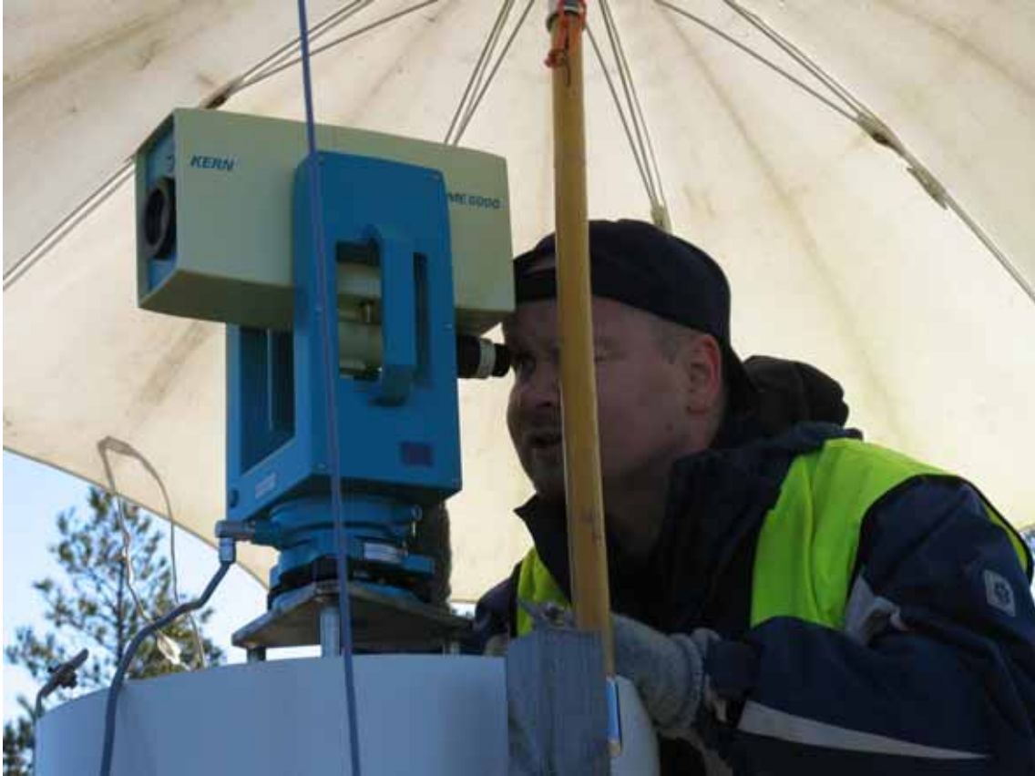
Figure 5-1. The mekometer Kern ME5000 at the pillar GPS7 during baseline observation on September 2007. (Photograph J. Puupponen 2007.)
