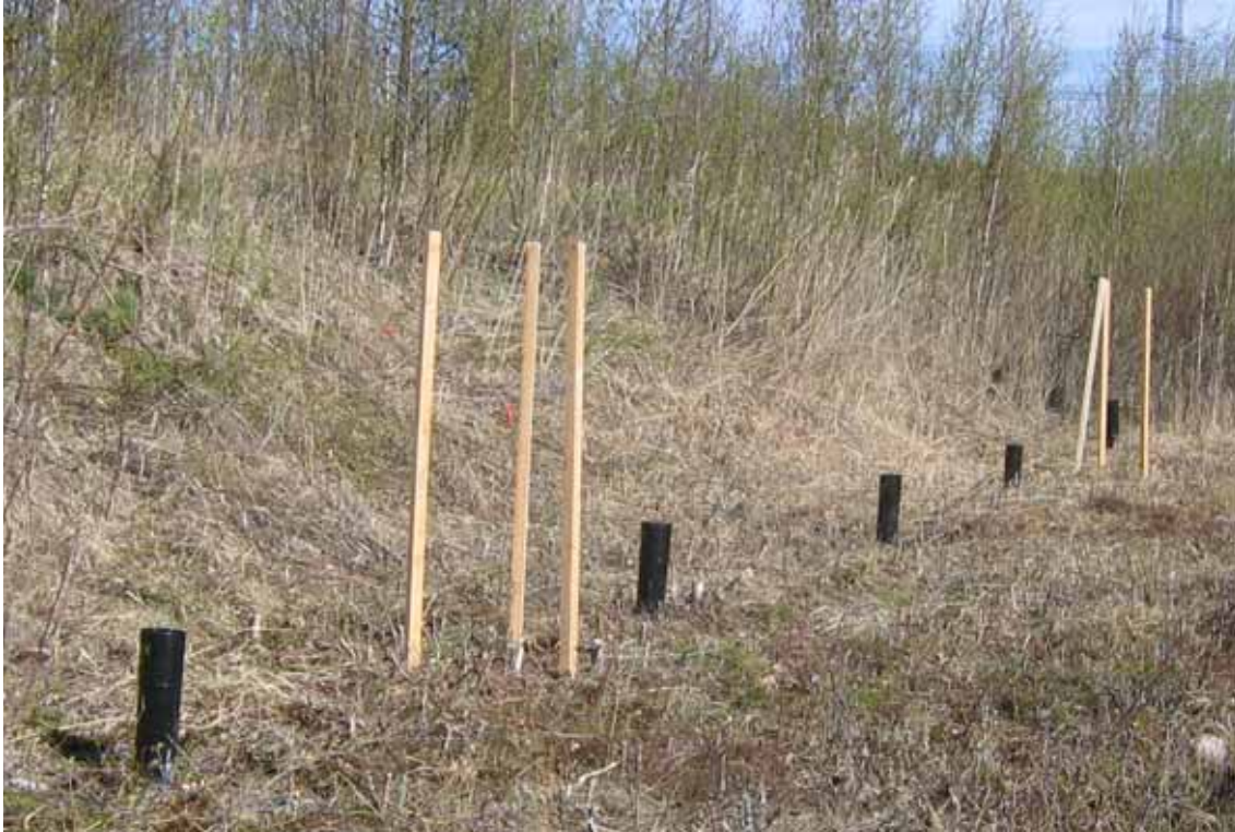
Figure 3. A new monitoring plot in an open area (MRK13) with five rainwater and two snow collectors was established in the vicinity of the Korvensuo freshwater reservoir in May 2009 (Photo: A. Ryyänänen/Metla, see also Figure 2).
