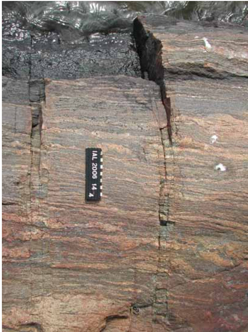
Figure 5. Small-scale joint clusters cross-cutting sheared, well foliated migmatites in shore outcrops on an island adjacent to the Olkiluoto peninsula (Photo 2006-14.4A from the Appendix "Outcrop Photographs" in Lindberg 2007, scale bar 15 cm).
