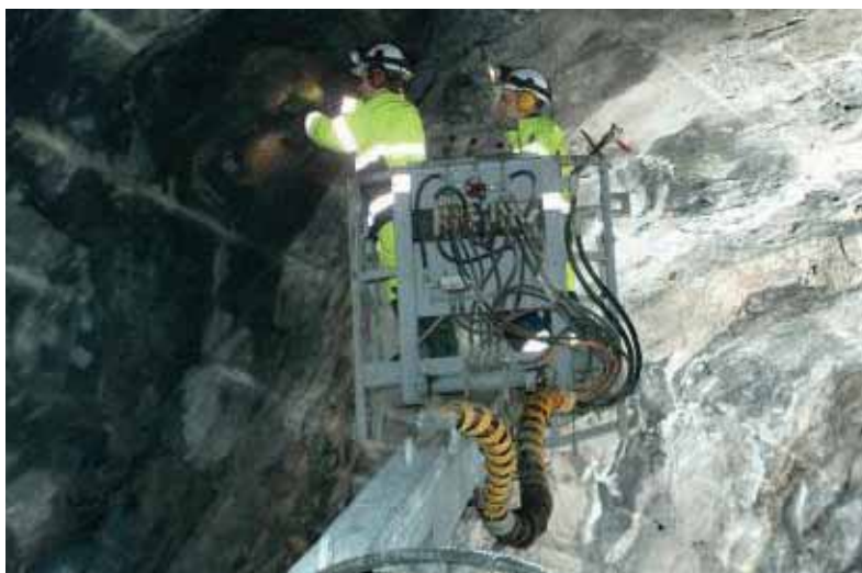
Figure 12. Systematic mapping of fractures, lithological contacts and foliation in the heterogeneous, migmatitic bedrock exposed in the ONKALO access tunnel, Olkiluoto. (Photo: Posiva).
