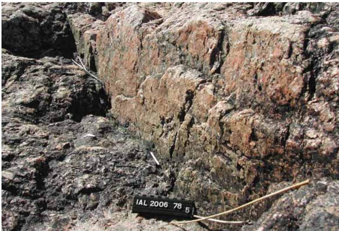
Figure 14. Slickenside fracture surface in a fault zone cutting altered pegmatitic granite in shore outcrops near Olkiluoto (Photo 2006-78.5B from the Appendix "Outcrop Photographs" in Lindberg 2007, scale bar 15 cm).
