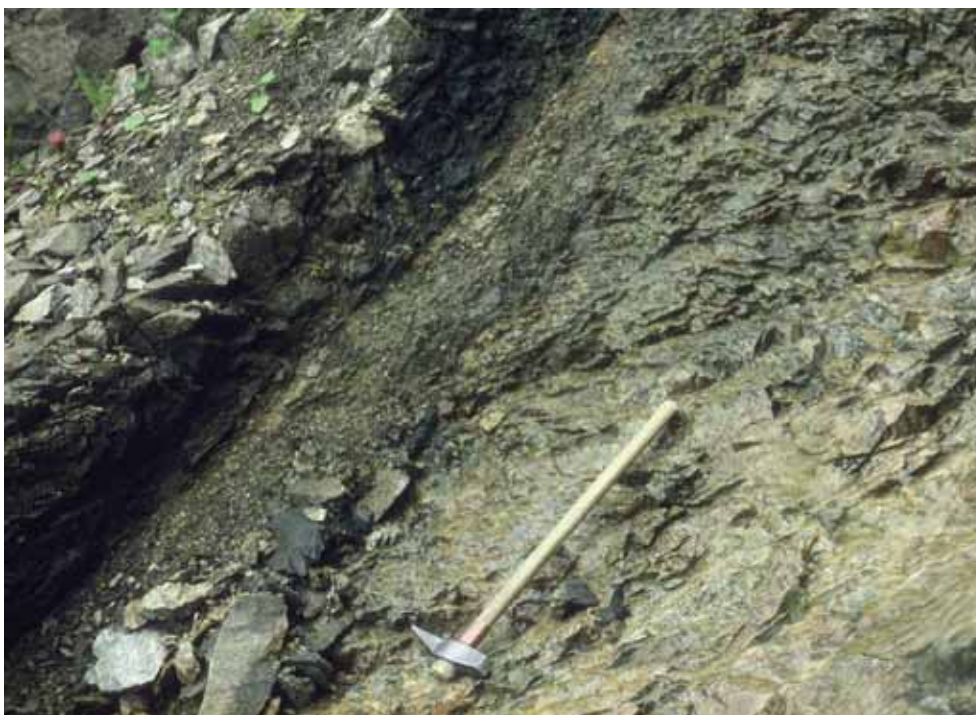
Figure 10. Fault gouge and incohesive fault breccia in the core of a small fault in migmatitic bedrock, Flatanger, west coast of Norway (Photo: A.G. Milnes).
