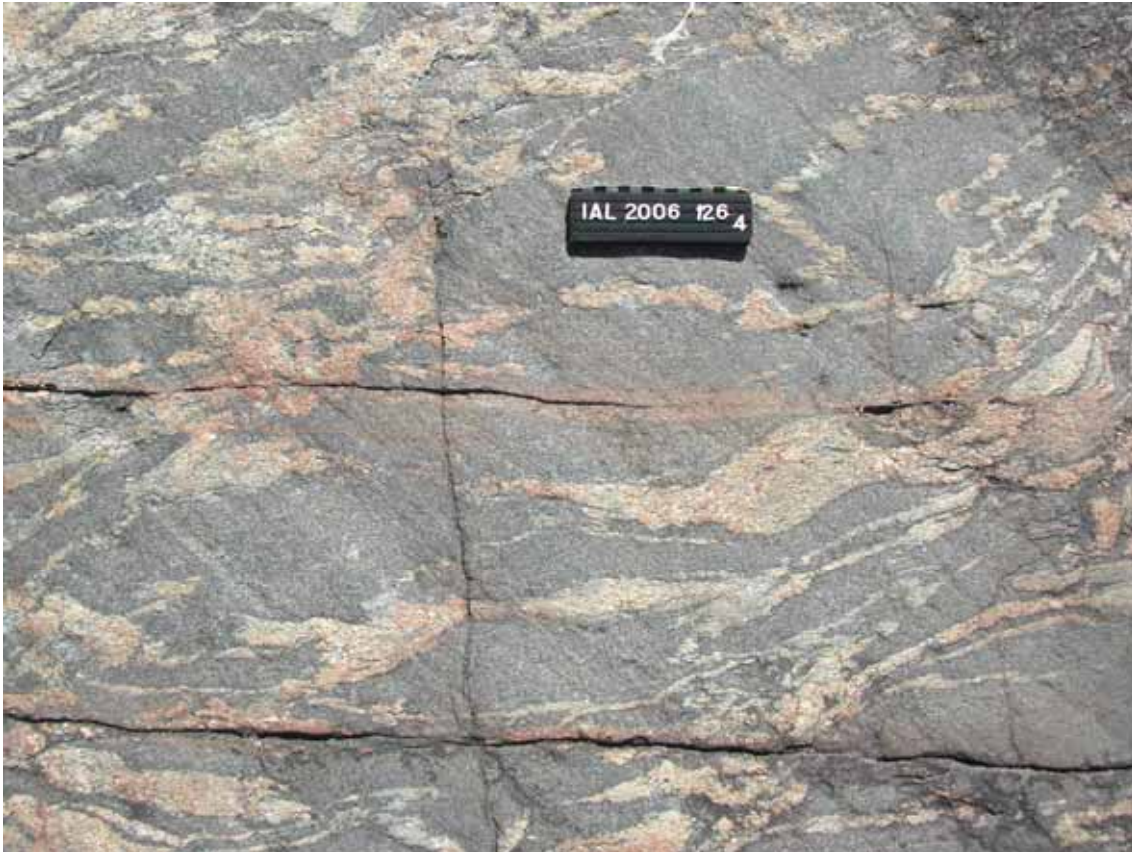
Figure 11. Migmatitic bedrock intersected by two sets of joints of different ages: the "E-W" joints show mineralization and wall-rock alteration, which is cut through by the younger, "N-S", unmineralized joints. Glacially striated shore outcrop near Olkiluoto (Photo 2006-126.4B from the Appendix "Outcrop Photographs" in Lindberg 2007, scale bar 15 cm).
