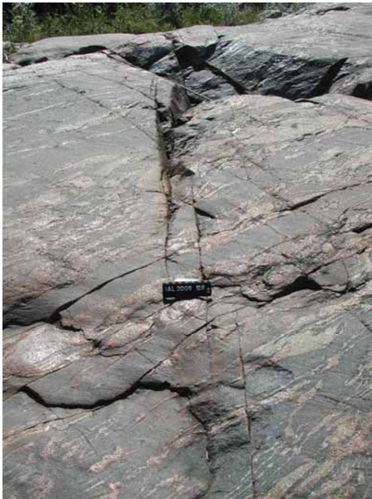
Figure 9. Migmatitic bedrock intersected by three sets of joints on a shore outcrop near Olkiluoto (Photo 2006-126.2A from the Appendix "Outcrop Photographs" in Lindberg 2007, scale bar 15 cm).
