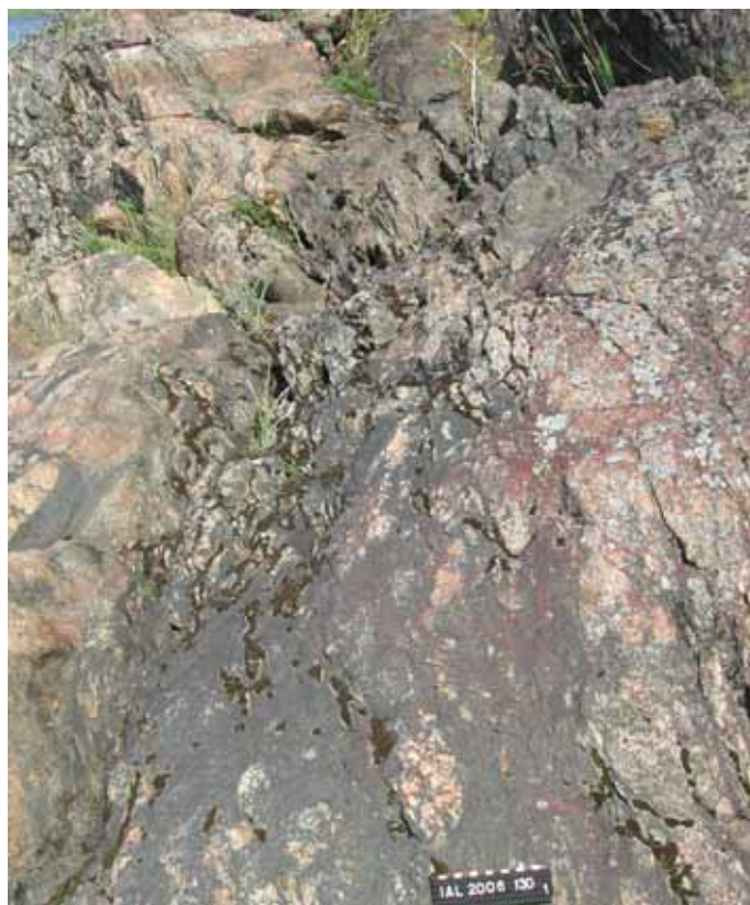
Figure 13. A semi-brittle deformation zone, later affected by brittle fracturing, intersecting and fragmenting migmatitic rocks in a shore outcrop near Olkiluoto (Photo 2006-130.1B from the Appendix "Outcrop Photographs" in Lindberg 2007, scale bar 15 cm).
