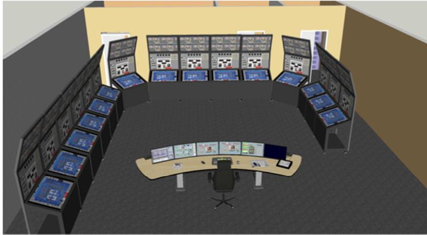
*FIG. 3. Proposed control room layout using glass top panels*
