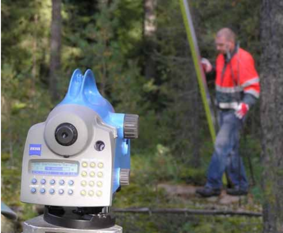
Figure 9. Bench mark interval has been measured and the levelling instrument Zeiss DiNi 12 and the second rod man will have a brake (Photo A. Hiironen).
