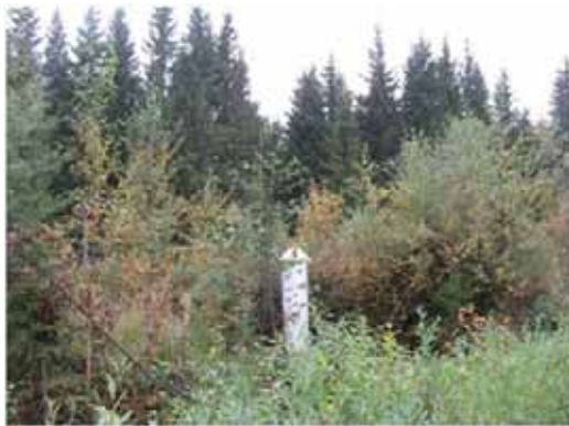
Figure 4-7. Forest growing is clearly visible in the NEU time series at GPS2 pillar (Kivetty).
