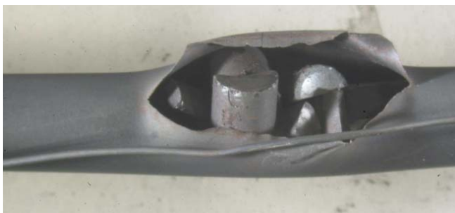
Figure 9. Tests in the Halden Reactor performed to investigate high burn-up fuel relocation during LOCA.
