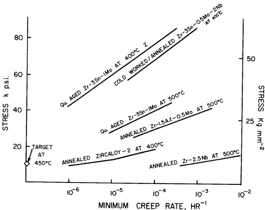
Figure 5 Stress Dependence Of Minimum Creep Rates For Complex Zr Alloys
