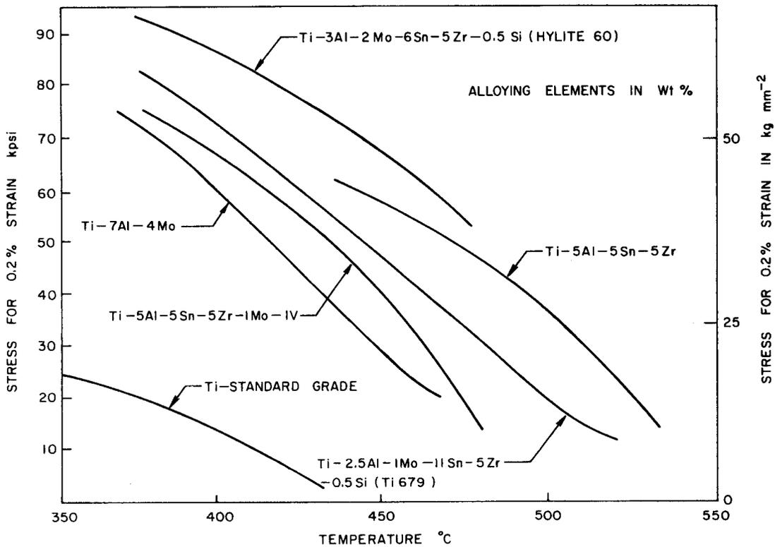
Figure 3 Stress To Give 0.2% Strain In 1000 Hours At 350-550°C In Titanium Alloys.
