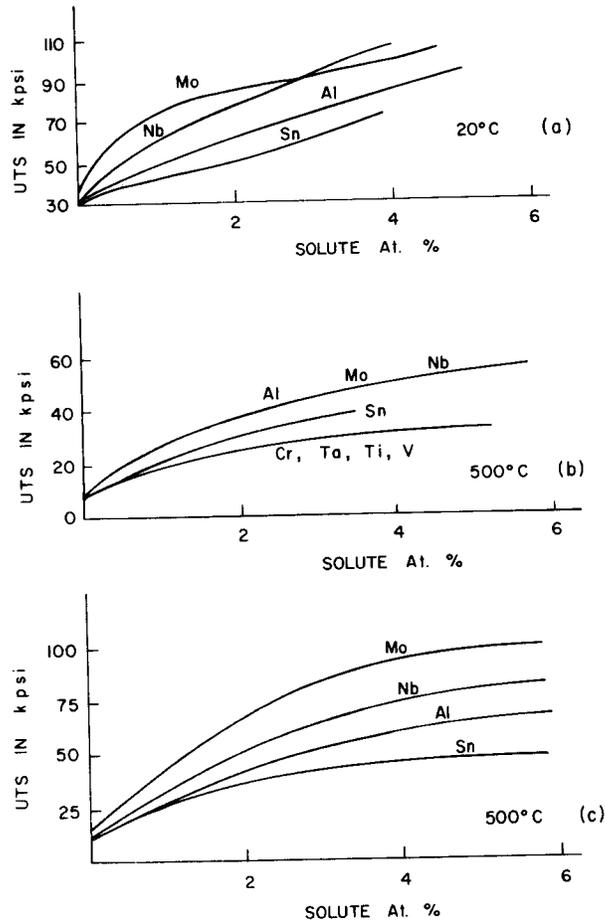
Figure 2 Strength Of Some Zirconium Alloys
