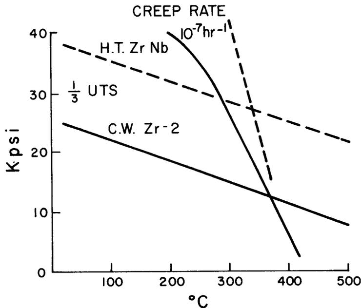
Figure 1 Design Stresses For Zr Alloys
