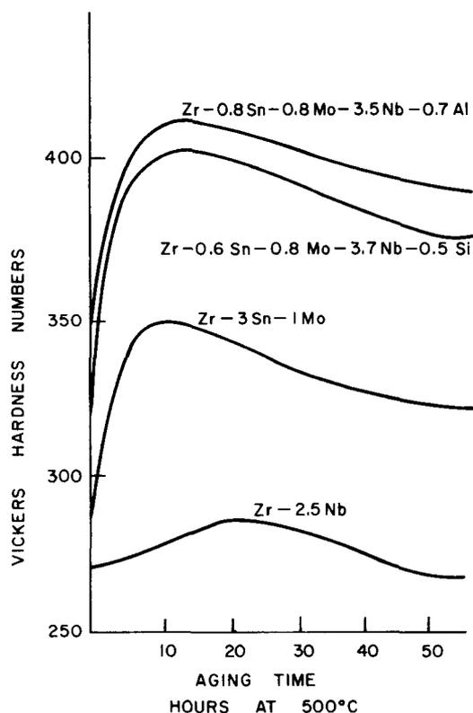
Figure 4 Age Hardening Of  $\beta$ -Quenched Complex Zr Alloys
