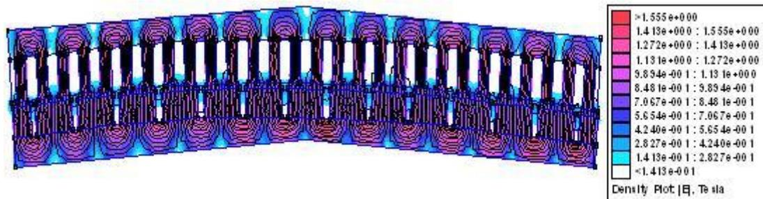
Fig. 6 The magnetic field map in no-load condition
