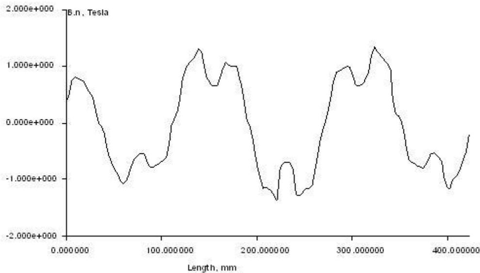
Fig. 10 The normal component of magnetic flux density in loaded condition
