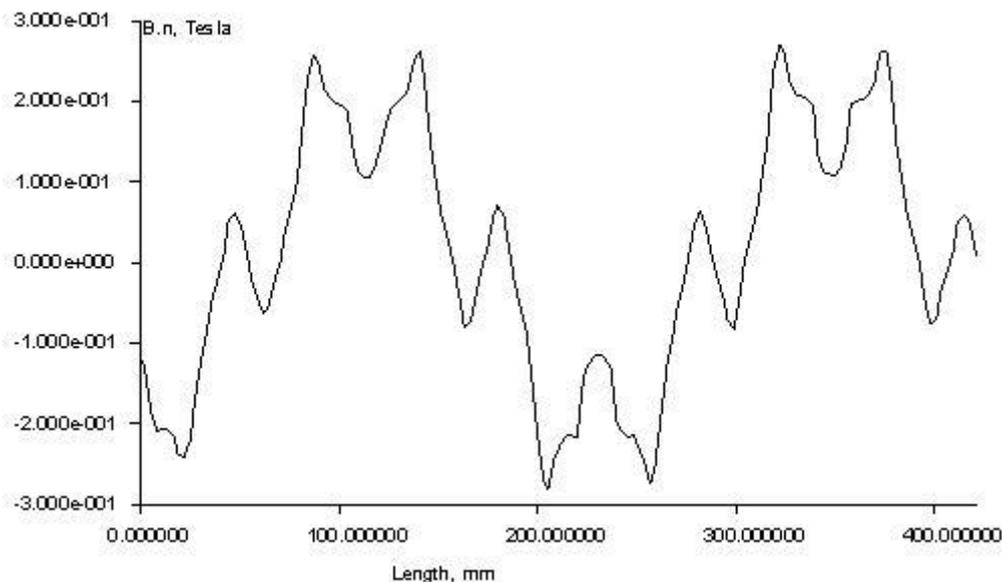
Fig. 13 The normal component of magnetic flux density for armature reaction
