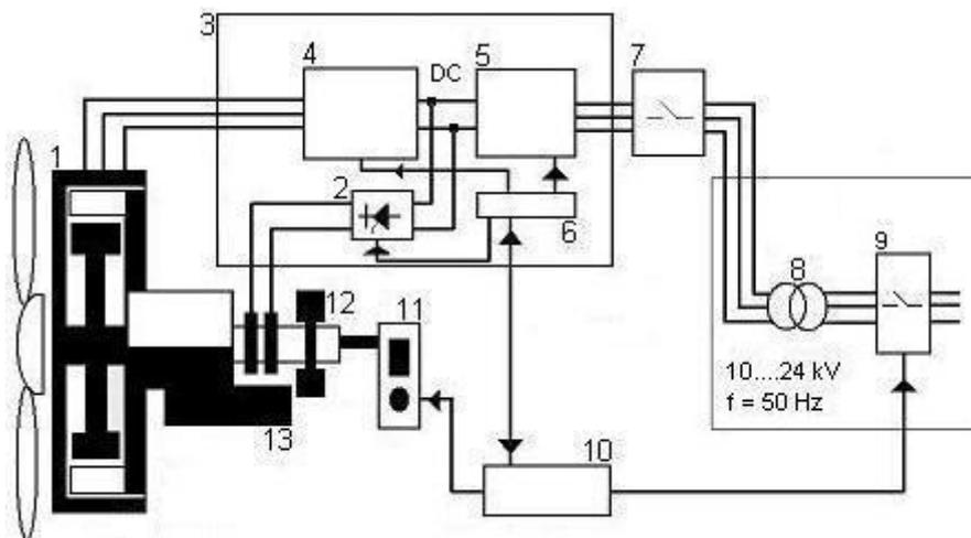
Fig. 1 Multi pole synchronous generator driven directly by the turbine
