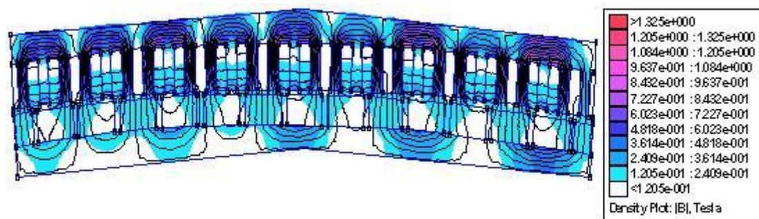
Fig. 12 The magnetic field map for armature reaction
