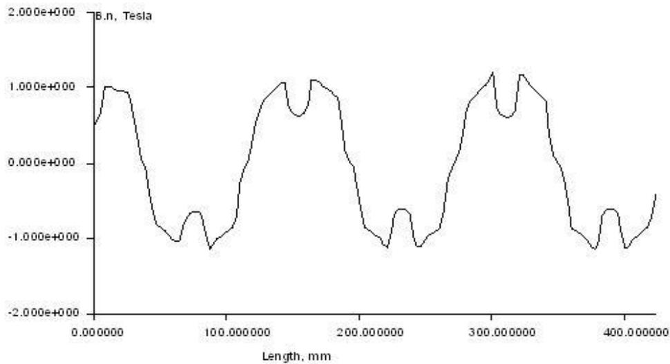
Fig. 7 The normal component of magnetic flux density in no-load condition
