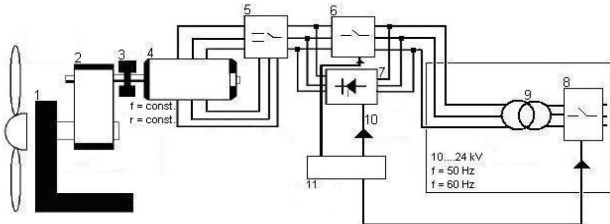
Fig. 2 Induction generator with squirrel cage
