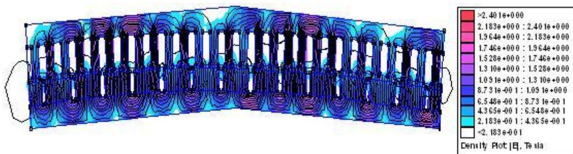
Fig. 9 The magnetic field map in loaded condition
