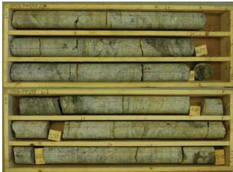
Figure 2-4. The ONK-PP269 drillhole core used for the DRA tests. The depth markings show that the core was obtained from 3 m to 7 m below the niche floor.
