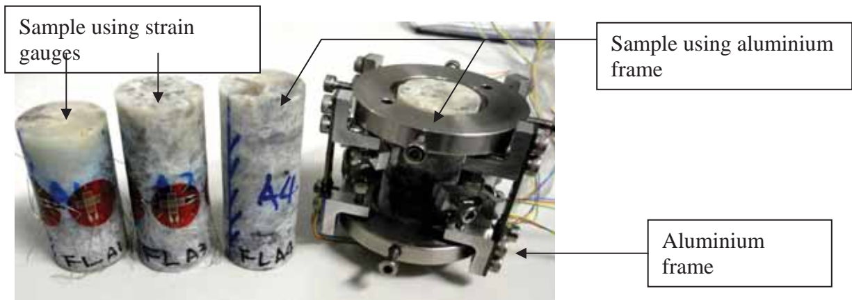
Figure 3-2. The sub-cores used for the DRA testing programme. The aluminium frame is equipped with four axial and two lateral strain gauges.
