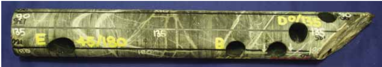
Figure 3-1a. Typical sub-core sample orientations and markup. The lines along the core have been measured from the bottom of core mark (BOC), which was marked as 0 degrees when looking downward on a core.
