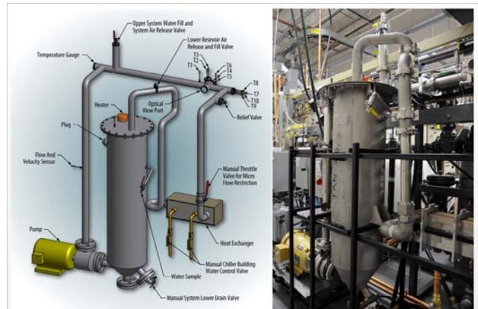
Figure 3: Diagram of the hot water corrosion flow test system and the assembled test equipment at INL; test samples are installed in the top leg of the flow loop at the optical view port position.
