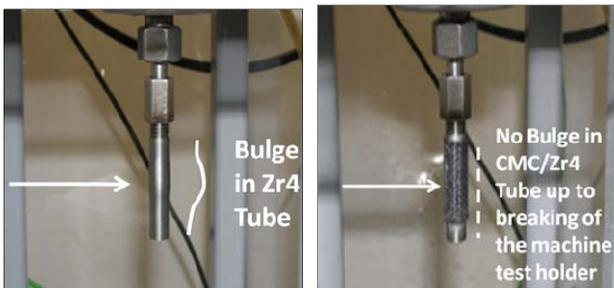
Figure 2: Halden Burst Testing of Zr4 Tube to Failure. Zr4 metal tube failed at 437 MPa (left). The INL hybrid cladding design shows no bulge at failure limit of sample holder at 460 MPa (right).
