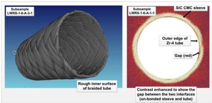
Figure 1: Three dimensional reconstruction of SiC CMC sleeve and fabricated hybrid tube geometry using 3D X-ray tomography techniques.
