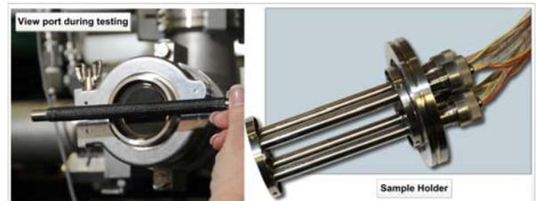
Figure 4: Photos showing the position of the sample during testing and the sample holder, which can hold up to four samples during testing
