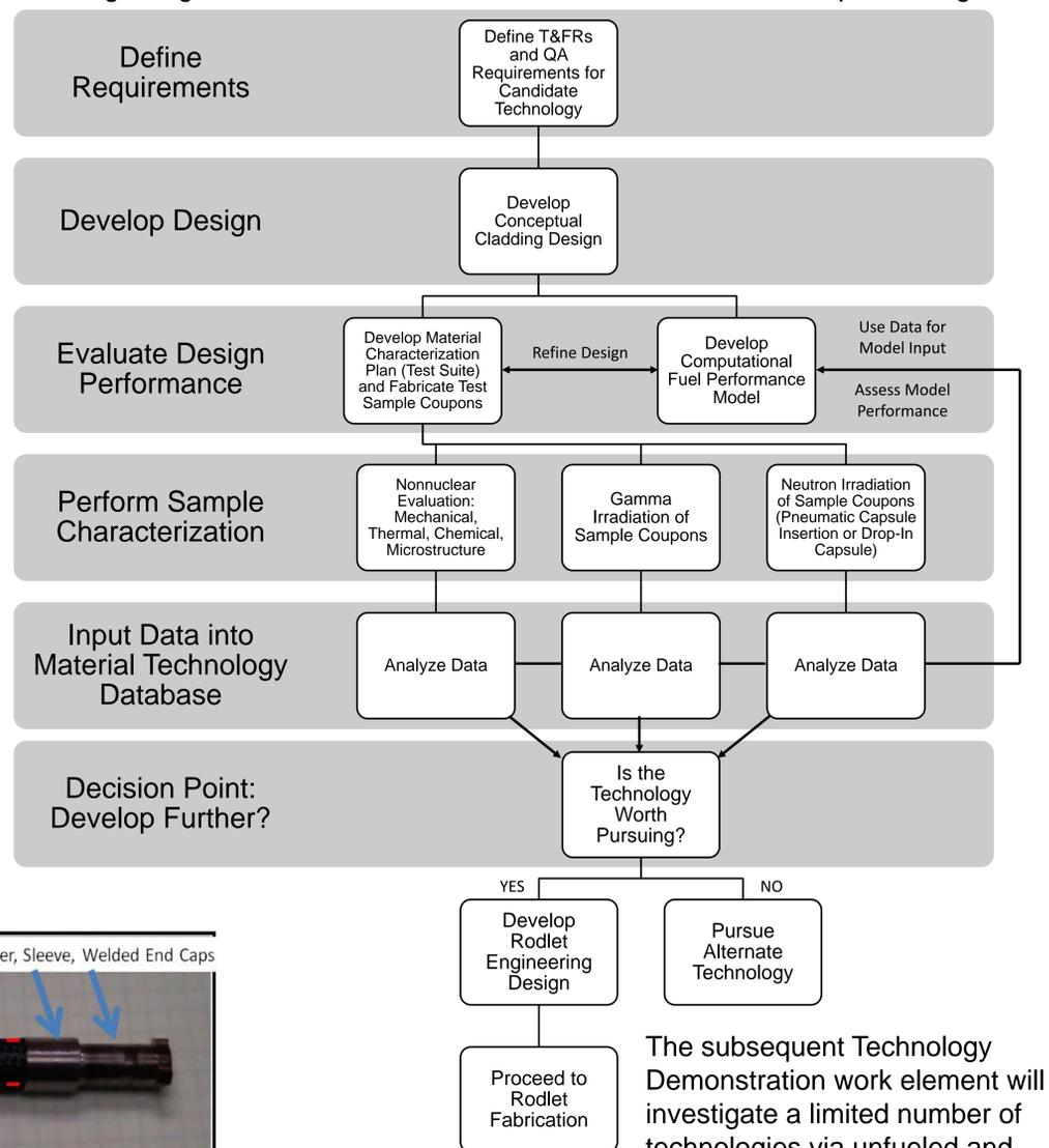
The subsequent Technology Demonstration work element will investigate a limited number of technologies via unfueled and fueled rodlet fabrication, characterization and irradiation at steady-state, transient and accident conditions.
