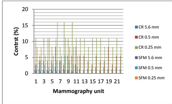
Figure 4. Contrast for details 5.6 mm, 0.5 mm and 0.25 mm size for screen-film and CR mammography units
