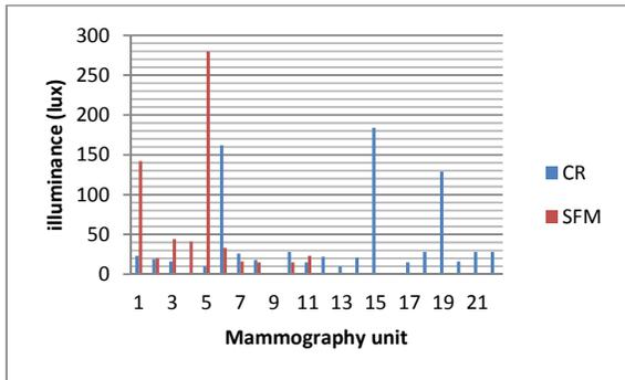
Figure 7. Ambient light level in viewing environment in mammography units equipped with screen-film and CR detectors
