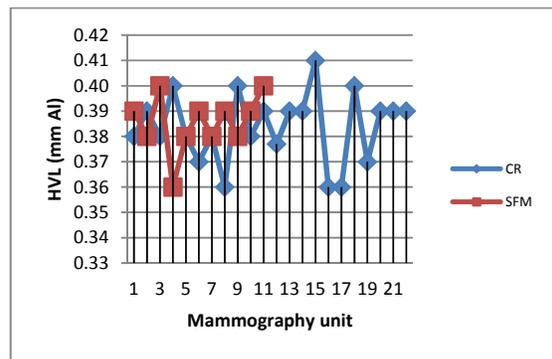
Figure 2. Half-value layer for Mo/Mo target/filter combination for screen-film and CR mammography units
