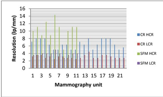
Figure 3. High and low contrast resolution for screen-film and CR mammography units
