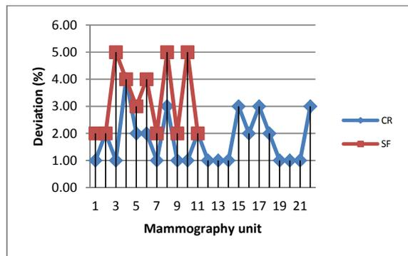
Figure 1. Tube voltage accuracy measure at 28 kV for screen-film and CR mammography units
