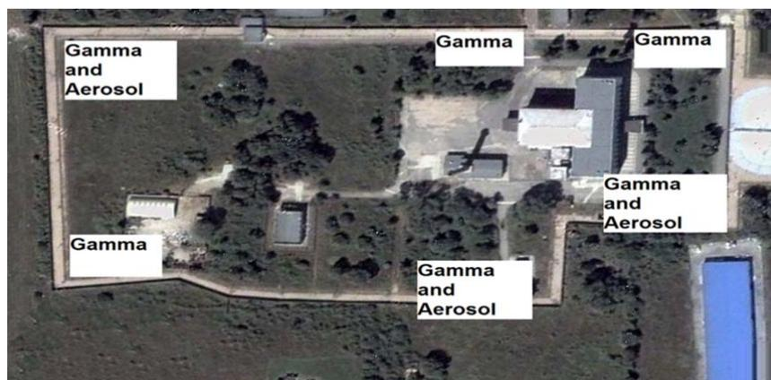
Figure 1. Scheme of radiation monitoring stations in IRT-Sofia
